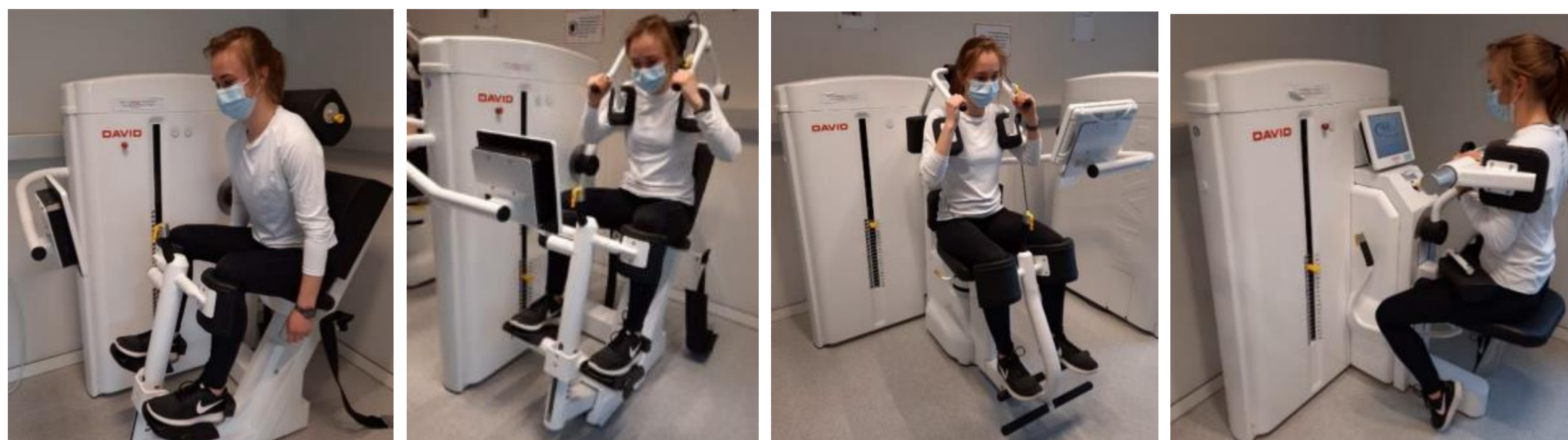
Figure 1 : David Back Dynamometers (David International Ltd., Vantaa, Finland) for trunk extension, flexion, rotation and lateral flexion respectively.
