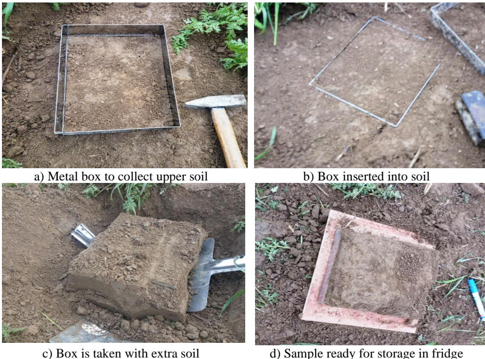
Figure 2-2 Photos showing sample collection using metal box from the field of study
