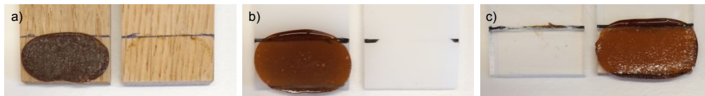
Figure S30. Photos of the representative adhesion failure after lap-shear tests of 50/50-MXDA when it was applied onto a) oak, b) PE-HD and c) PMMA.
