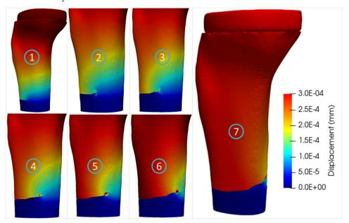
Figure 12. Crack propagation in the tibia bone model with implant of the 27-year-old female.
