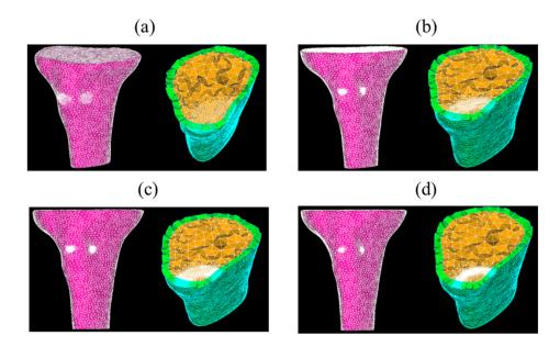
Figure 5. Four meshes of the tibia model without implant—coarse (a), medium (b), fine (c), and very fine (d) meshes.
