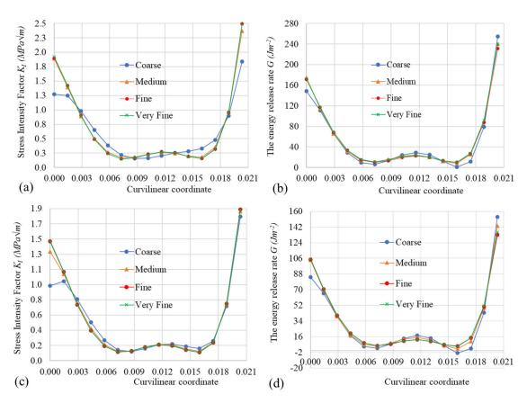
**Figure 7.** Mesh size effect on the values of  $K_I$  and of G versus the curvilinear coordinate along the crack tip—the tibia model without the implant  $(\mathbf{a},\mathbf{b})$  and the tibia model with the implant  $(\mathbf{c},\mathbf{d})$ .
