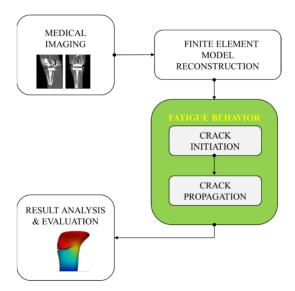
**Figure 1.** Overview of the developed modeling and simulation workflow for analyzing the tibia crack propagation.
