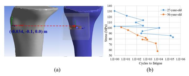
**Figure 3.** Location of the crack initiation based on the clinical observation (**a**) and the Stress-Cycles to fatigue diagram (the so-called SN curve) from the accumulation of fatigue micro-damage in the human cortical bone of two different ages used in the age-related critical point identification process extracted from [20] (**b**).
