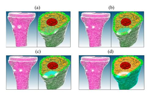
**Figure 6.** Four meshes of the tibia model with implant (TKR model)—coarse (a), medium (b), fine (c), and very fine (d) meshes.
