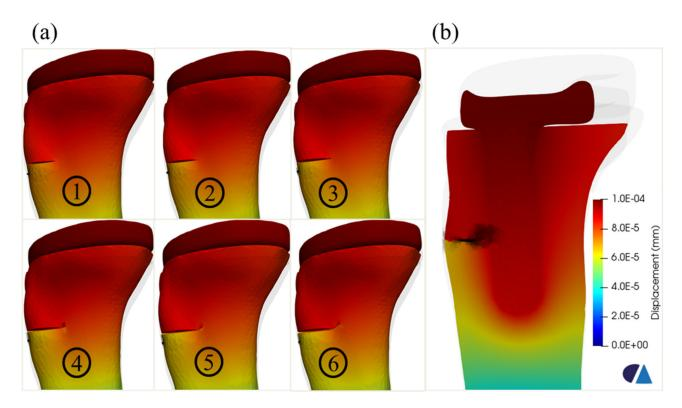
**Figure 9.** Crack propagation in the tibia model with implant—different steps (**a**) and a slicing surface along the implant in the last step (**b**).
