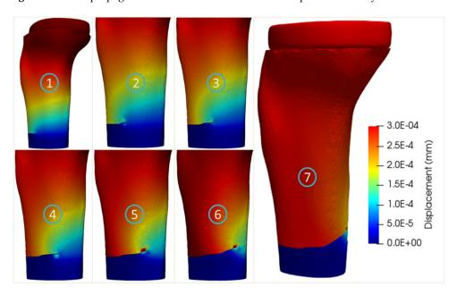
Figure 13. Crack propagation of the tibia bone model with implant of the 56-year-old female.
