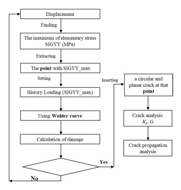
Figure 4. The flow chart of the age-related critical point identification process.
