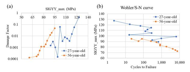
Figure 11. The fatigue damage curve (a) and S-N curve (b) for two age-related tibia models with implant.
