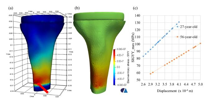
**Figure 10.** Maximum stress location (red arrow) of the 56-aged model, (**a**) the distribution of the stress component SIGYY of the 56-aged model (**b**), and the history of SIGYY\_max versus the displacement at the maximum stress location (**c**).
