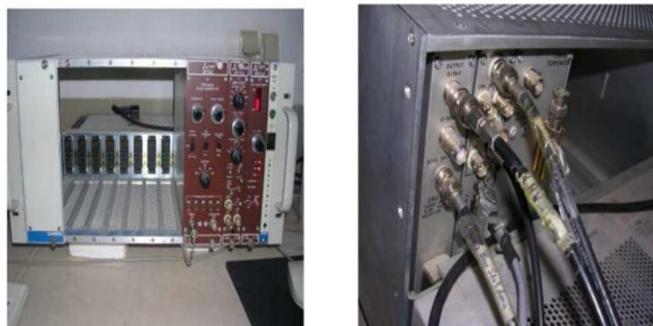
**Figure 3-7:** Canberra Amplifier - Nuclear Instrument Module (NIM) of the detection system used.
