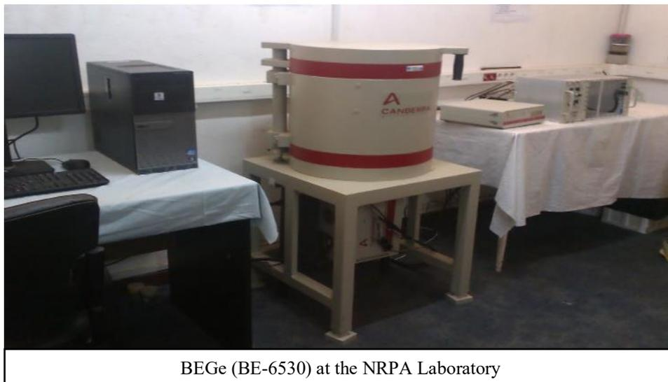
**Figure 3-2:** Broad Energy Germanium detector (BE 6540 model) used in Cameroon
