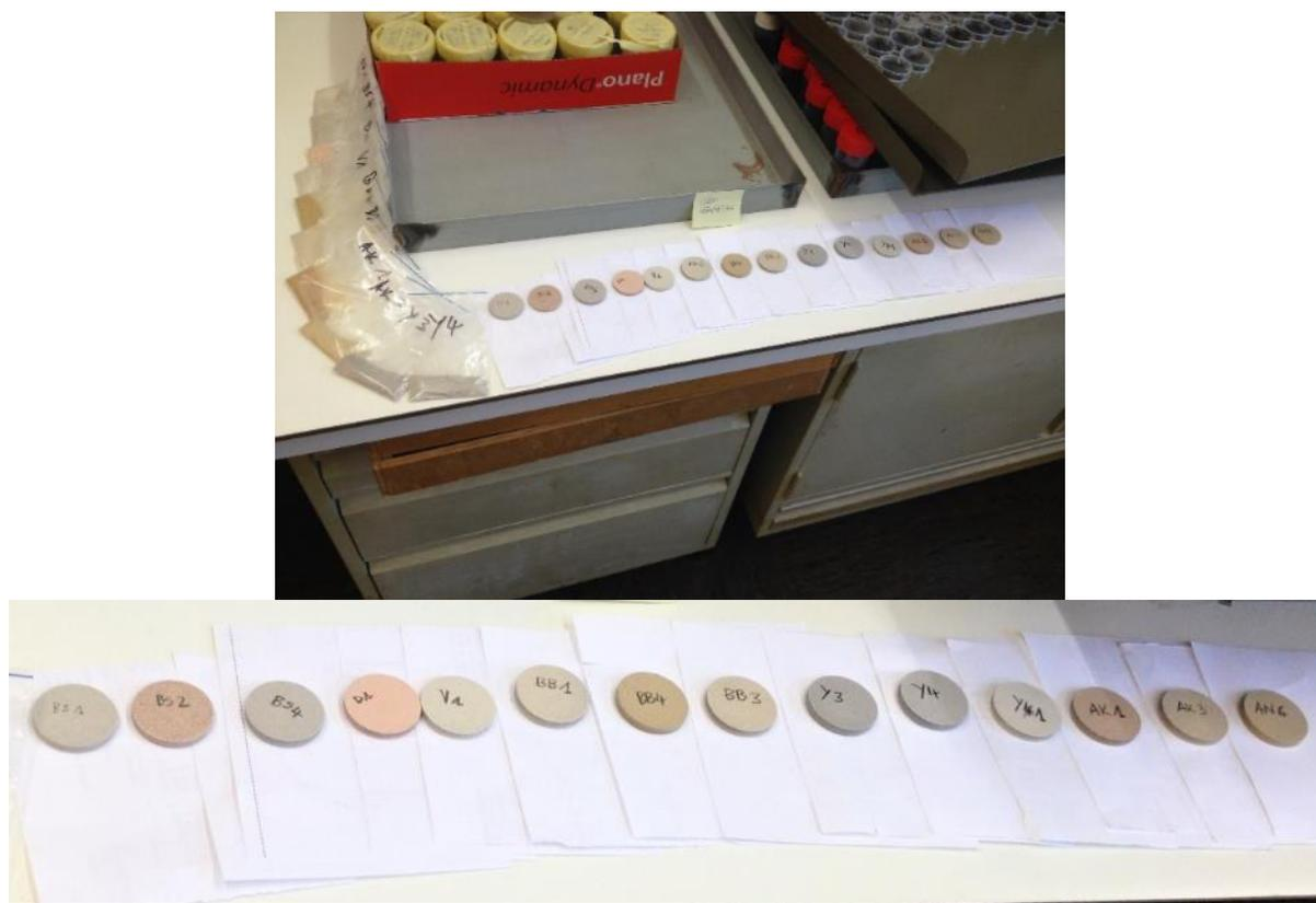
**Figure 5-3:** Pressed pellet preparation process for EDXRF measurement. All samples were labelled, and the labelling process took place at each step of the preparation as well. The measurement (irradiation) was performed on the sample side facing the ground without any labelling mark. Different colors of the pressed pellet represent the color of the sample (sand present in chapter 4).
