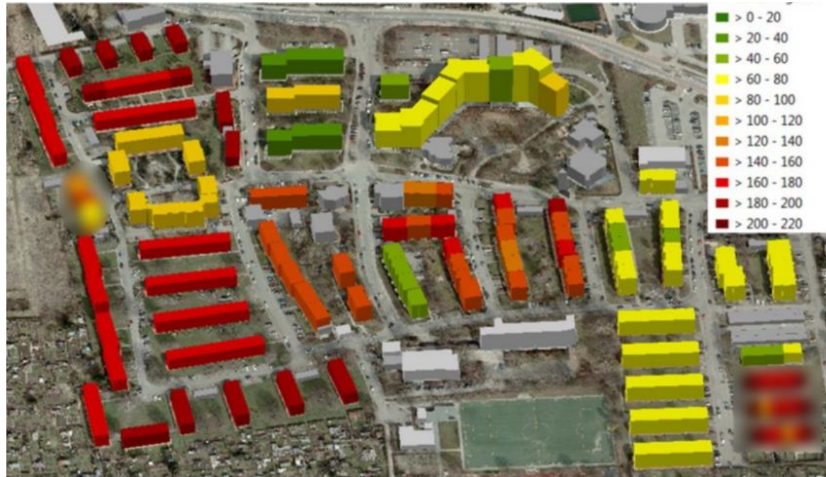
Example of using a CityGML to Model Building's Energy Demand in Ludwigsburg — Grünbühl (The energy modeling is calculated with SimStadt2 software)
