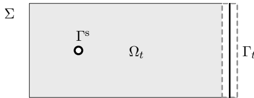
Figure 2.13: Example of a two-dimensional domain \Omega_t with source boundary \Gamma_s and moving scatterer boundary \Gamma(t) .
