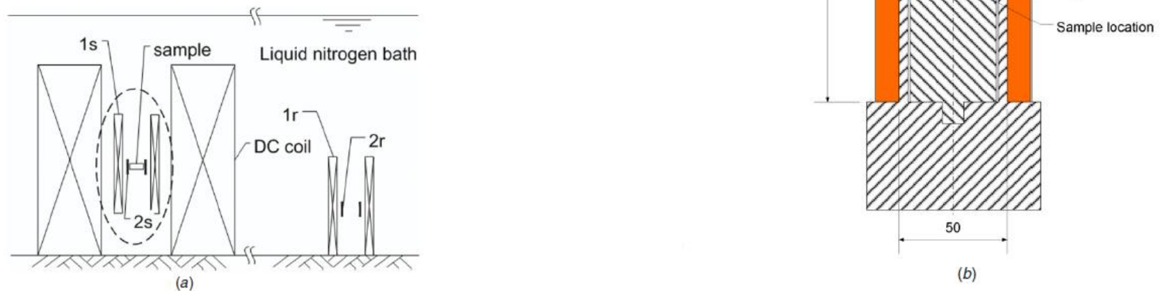
Figure 1. (a) Schematic illustration of the geometrical arrangement of the coils used for the ac susceptometer. The primary coil consists of two separate coils, one containing the sample (coil '1s') and one used for reference (coil '1r'). Coil '1s' can be inserted in a large coil that can generate a dc magnetic field. Primary coils '1s' and '1r' contain their own secondary coil, '2s' and '2r', respectively. (b) Cross-section of the part of the susceptometer containing the sample illustrating the geometry of the primary coil '1s' and the secondary coil '2s'. All dimensions are given in mm. The sample, located in a vacuum vessel, is centred in the secondary coil '2s'. The reference coils ('1r' and '2r') are identical to those shown in figure 1(b).
