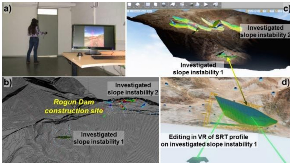
Fig. 5. Rogun site in virtual reality. a) Researcher visiting the site in VR. b) General semi-transparent surface view showing subsurface profiles. c) Illuminating collected subsurface data near the Rogun site inside the virtual environment. d) Visualisation of geophysical (SRT) profile edited (placed at correct location) in VR. For this site also simulations of rock falls were completed in 2D with the UDEC (ITASCA) software. Final results are included as section in the virtual model (see Fig. 4d).
