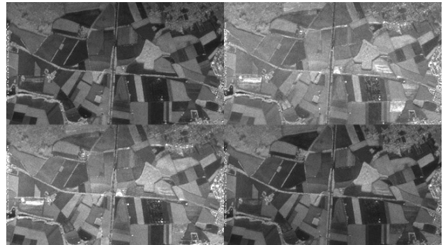
Figure 5 Amplitude images of bistatic acquisition in the 4 polarization channels, flight M4. From top left to bottom right: HH, HV, VH and VV.
