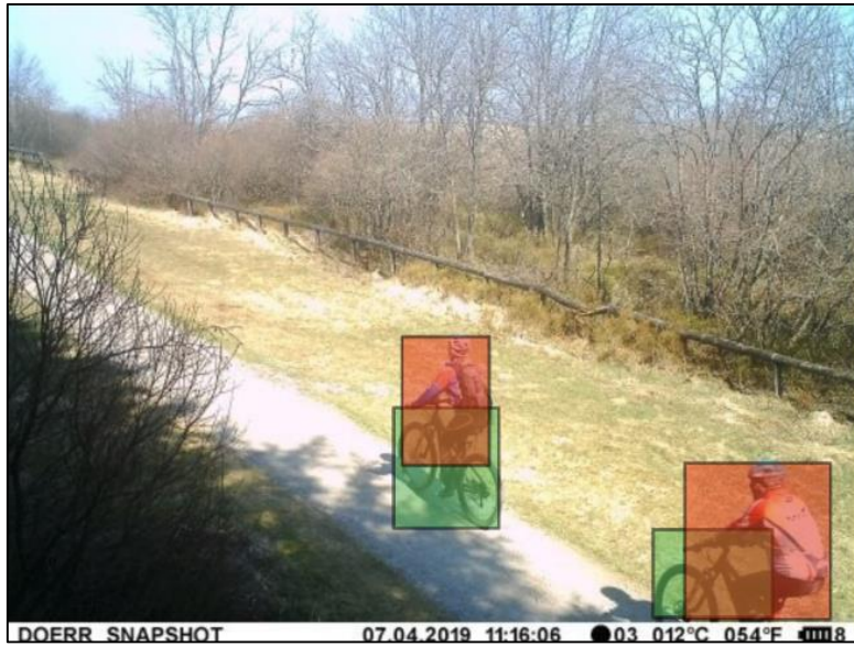
Figure 5. Example of a processed image with bounding boxes for each detected/identified object, in this case two persons (red) and two bikes (green)
