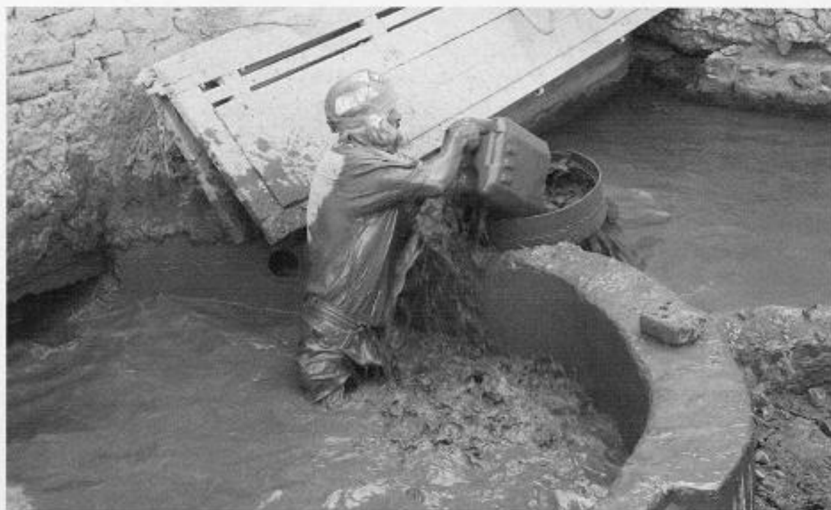
Figure 6. Workshop 1: clay basin in the courtyard. Bailing the clay and water with a bucket out of the water basin and throwing it through a sieve into the adjacent basin.
