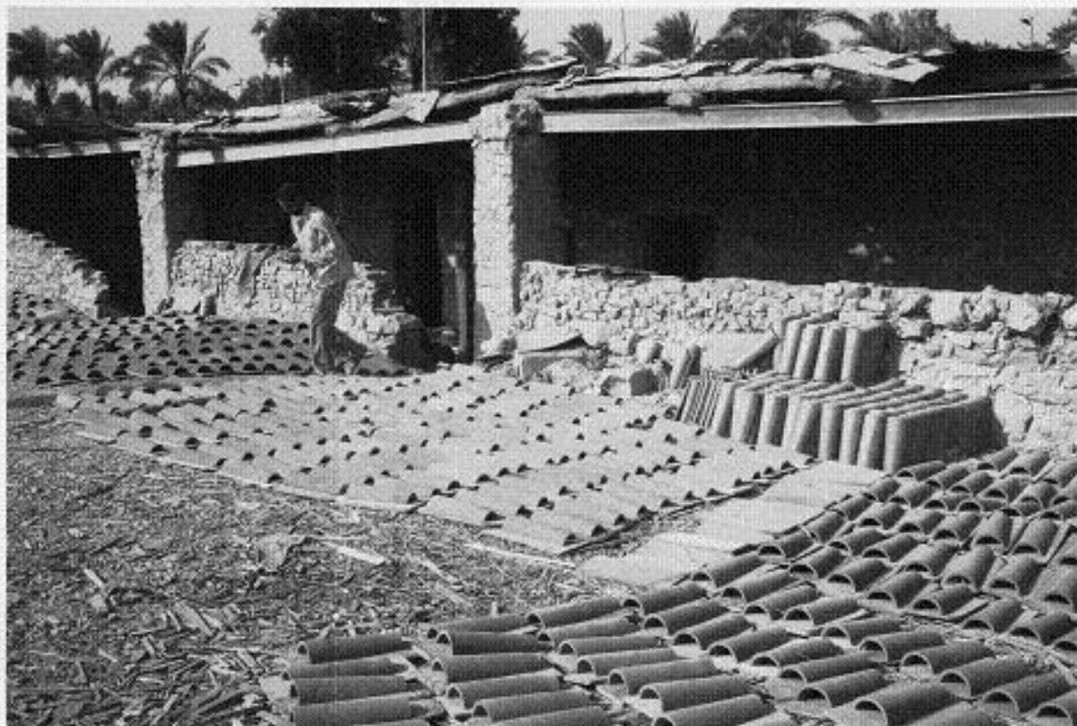
Figure 13. The terrain in front of workshop 3, where the roof tiles are laid out to dry.
