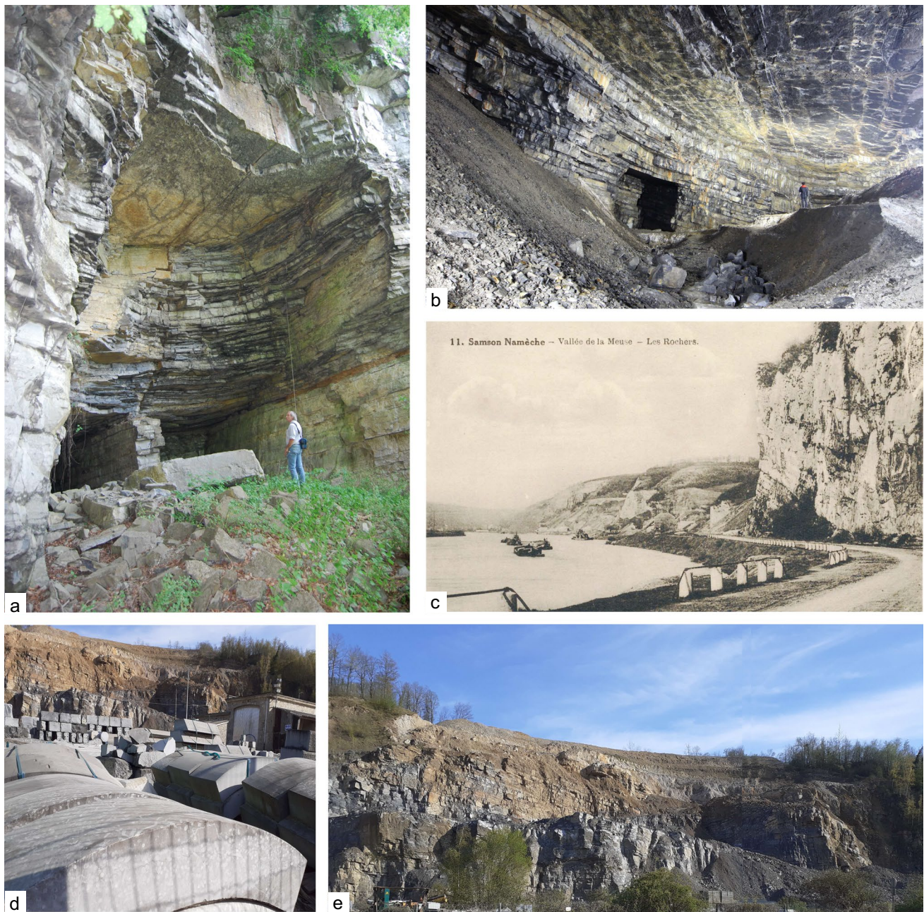
Fig. 8 Examples of ‘Pierre de Meuse’ quarries. a Lives quarry (Namur) with exposure of thin-bedded limestones of black marble quality (‘Marbre Noir de Namur’). b underground quarry of the Fond d’Arquet; note that the quarry has been partially filled with stone debris deriving from limestone production and lime burning (cour-
