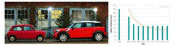
Figure 6. The same model has doubled in weight after thirty years of improvements in energy efficiency. The thickness of polysilicon wafers used in solar panels shows a downward trend from  $300\mu m$  down to  $160 \mu m$ .
