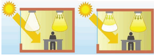
Figure 1.8: Lighting dimming system based on daylight management cell (Reiter and De Herde 2004, 265).
