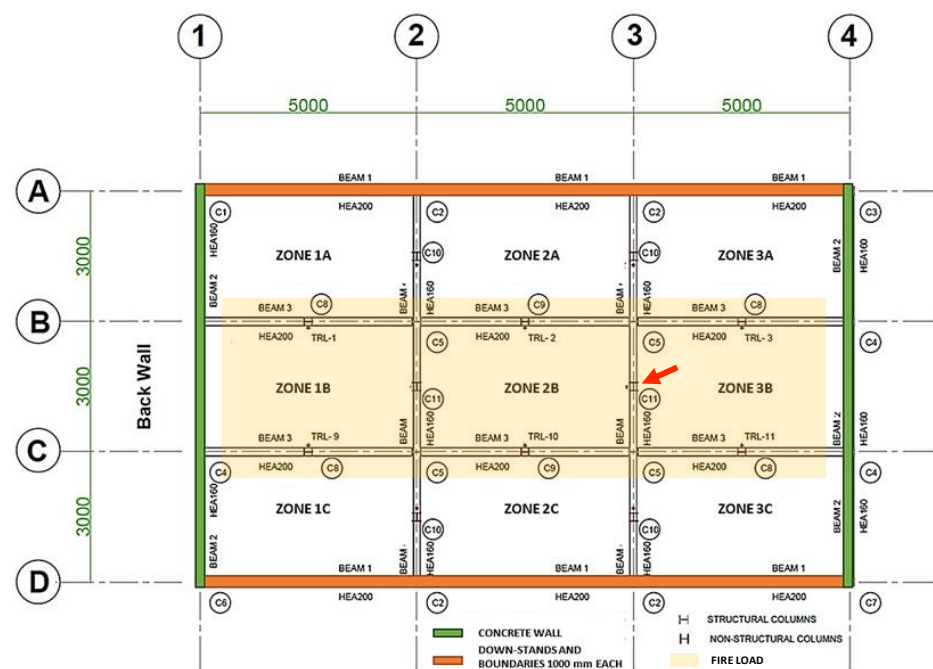
Figure 9. Layout plan of the test compartment, of the fire load and of the steel columns with considered column C11 highlighted (dimensions in mm) [28].
