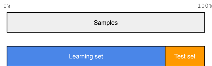
(A) Illustration of the train/test split method: a subset of data is kept for unbiased estimation.
