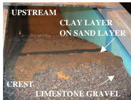
**Figure 3-3 : System of watertightness**
