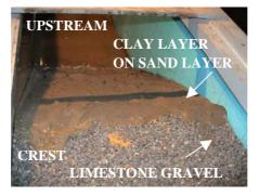
Figure 3-3 : System of watertightness
