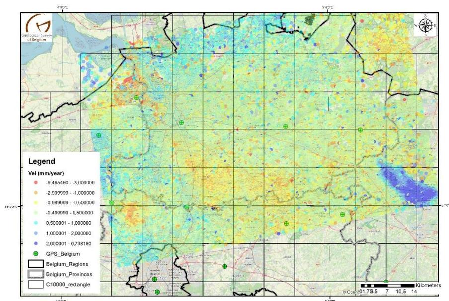
**Figure.** PSInSAR data showing the average LOS velocities (in mm/year) from Sentinel-1A ascending scenes (2016-2020) covering a large area in Flanders (between Brussels and Antwerp). Red colours indicate land subsidence areas while the blue colours indicate uplifting ground deformations. Green circles are the GNSS stations located in that area.
