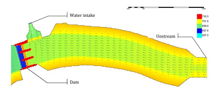
Figure 1: Bathymetry of the downstream part of the reservoir and location of the dam. Colour scale refers to the bottom elevation (m) while arrows show the velocity direction
