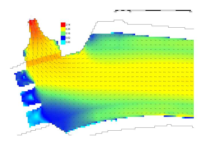
Figure 2: Flow field in the vicinity of the dam, computed with the k- $\square$  turbulence model and a grid resolution of 1 m by 1 m. Colour scale refers to the velocity magnitude (m/s) swhile arrows show the velocity direction.
