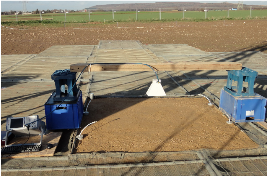
Figure 5.2: Picture of the VNA and radar antenna fixed at about 0.35–0.40 m above the sand surface.
