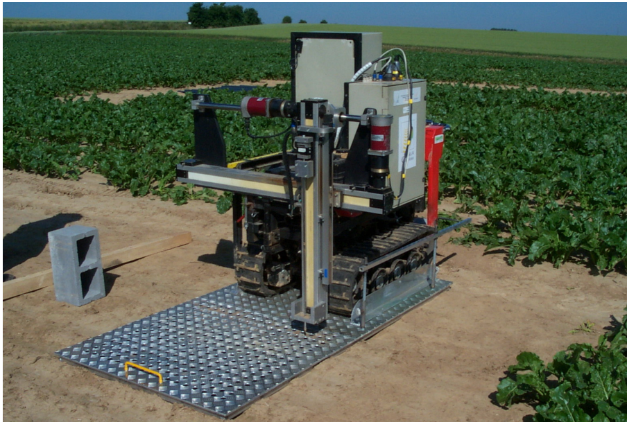
Figure 4.5: Fully automated penetrometer used for the soil strength measurements.
