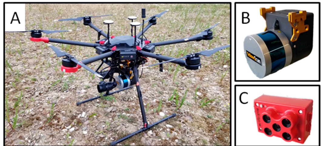
Figure 1. (A) The DJI Matrice 600 used in the study with (B) the YellowScan Surveyor LiDAR mounted below. In addition, the (C) Micasense RedEdge-M multispectral sensor that was used on a separate DJI Matrice 600.
