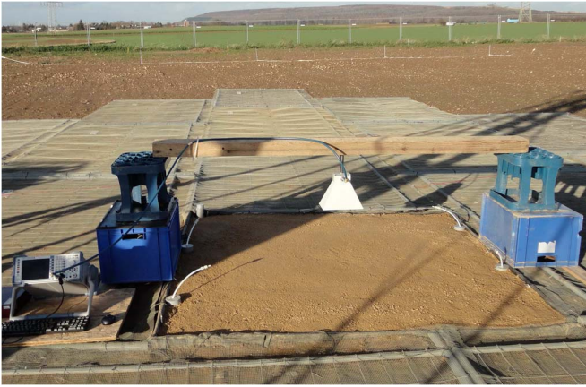
Fig. 2. Picture of the radar horn antenna connected to a vector network analyzer and fixed about 0.40 m above the sand surface.
