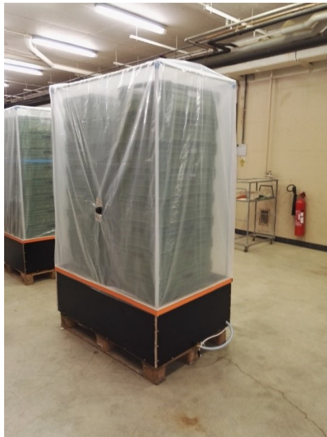
Figure 3-1. Picture of one experimental chamber (0.8 m x 1.2 m x 2.0 m) with a total capacity of 200 kg of potatoes.
