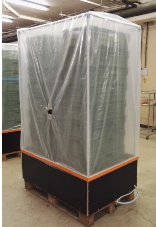
Figure 4-1. Automated experimental unit manufactured by Agroscope, which allowed potatoes to be treated independently in the same cold room. (Photo: Margot Visse-Mansiaux, Agroscope)
