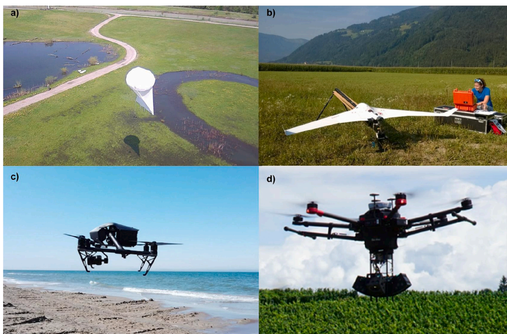
Fig. 1. Different platforms and sensors in UAS surveys; a) Lighter-Than-Air Helikite Balloon with Sony A7RII used for renaturation monitoring; b) BRAMOR ppk Fixed-Wing with Micasense Red Edge used for riparian vegetation monitoring; c) DJI Inspire 2 with zenuse x5s RGB camera, used for shallow water vegetation and beach cast monitoring (Palanga, Lithuania), and d) Leica Aibot AX 20 with multidirectional sensor prototype (5 Sony ILCE-QX1 RGB sensors for capturing NADIR and 4 oblique images). (For interpretation of the references to colour in this figure legend, the reader is referred to the web version of this article.)
