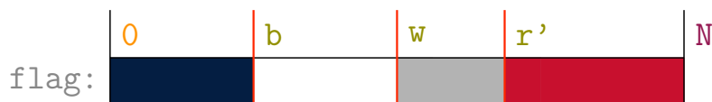
Figure 2.31: DUTCHFLAG problem: graphical weakest precondition for the Red area. In order to restore the Loop Invariant, if r is decreased, one should ensure that \text{flag}[r-1] is Red . That is the case if \text{flag}[w] is Red before swapping w and r-1 positions.
