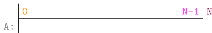
Figure 2.13: Pattern for Graphical Loop Invariant involving an array A of size N
