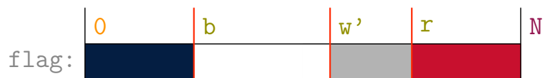
Figure 2.30: DUTCHFLAG problem: graphical weakest precondition for the White area. In order to restore the Loop Invariant when w is increased, \text{flag}[w] must be White .
