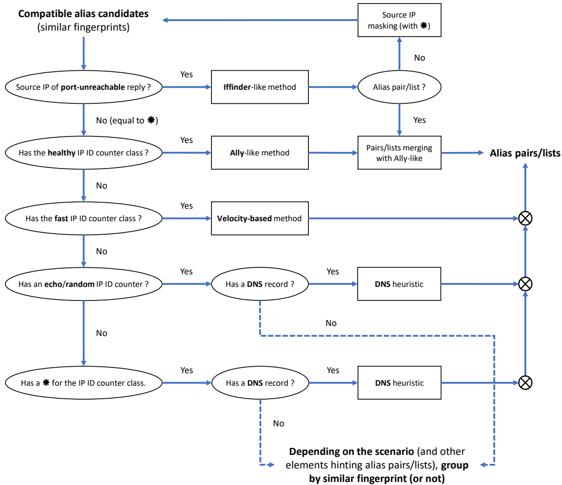
Figure 3.2: Practical selection of an alias resolution method as a flow-chart.
