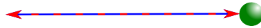
Figure 7.6 – Example of a self-retraced path. Those paths consist in paths that are backreflected at the first scattering event that takes place in the disorder potential. Obviously, such a path is identical to its time-reversed counterpart and hence do not enter in the Cooperon contribution that gives rise to coherent backscattering.
