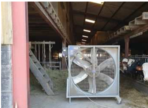
Figure 10 – Temporary fan used in case of high temperature to ensure a proper ventilation in the stables (with the courtesy of Dr Olivier Vandemaele, private vet practitioner, 2021)
