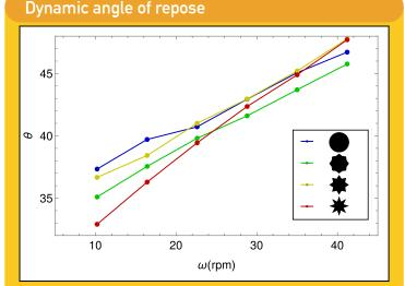
Higher dynamic angle of repose for irregular grains at high rotation speeds.
