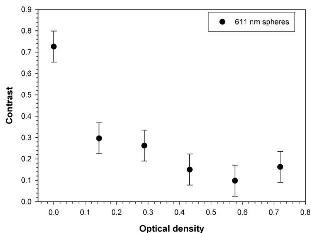
**Fig. 5** Contrast of the shearographic fringes versus optical density for different scattering phantoms composed of silica spheres ( $d=611$  nm) in suspension in distilled water.
