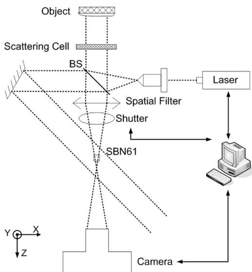
**Fig. 6** Experimental setup for photorefractive holography.
