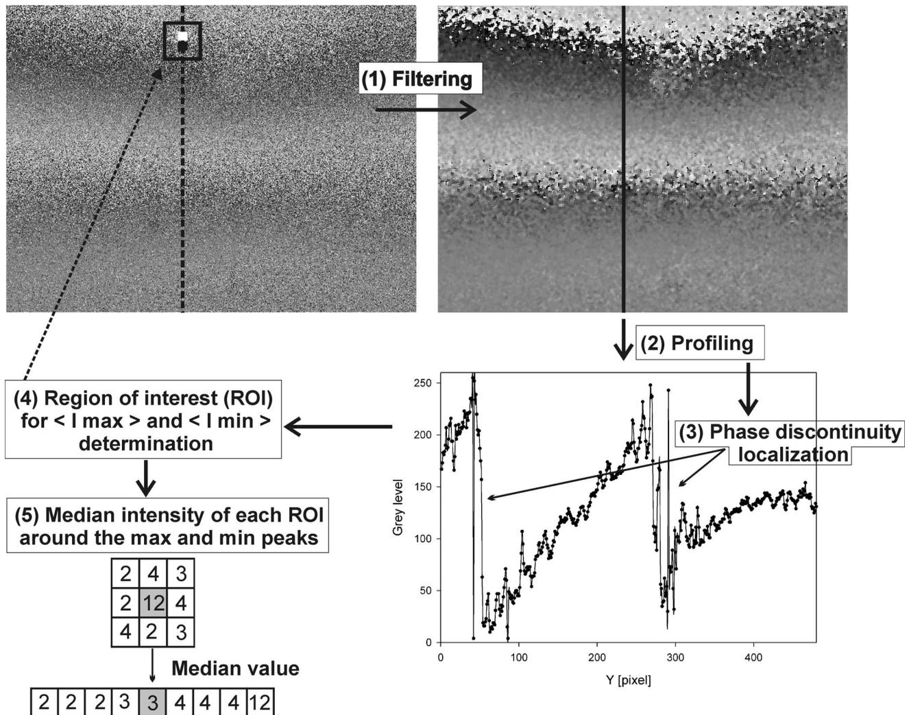
Fig. 4 Steps involved in the determination of  $\langle I_{\max} \rangle$  and  $\langle I_{\min} \rangle$  from the shearography phase maps.
