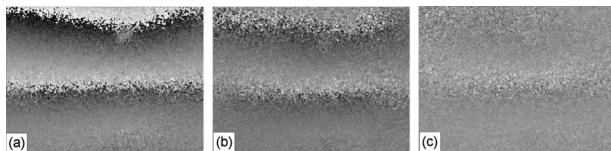
**Fig. 3** Wrapped differential phase maps ( $5 \times 5$  median filtered) obtained with the shearography setup. (a) Without a scattering cell; (b) with a scattering cell: OD=0.144; (c) with a scattering cell: OD=0.576.
