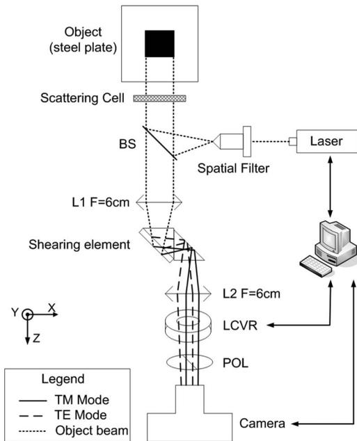
**Fig. 2** Experimental setup for shearography. The black square corresponds to the imaged area on the steel plate.
