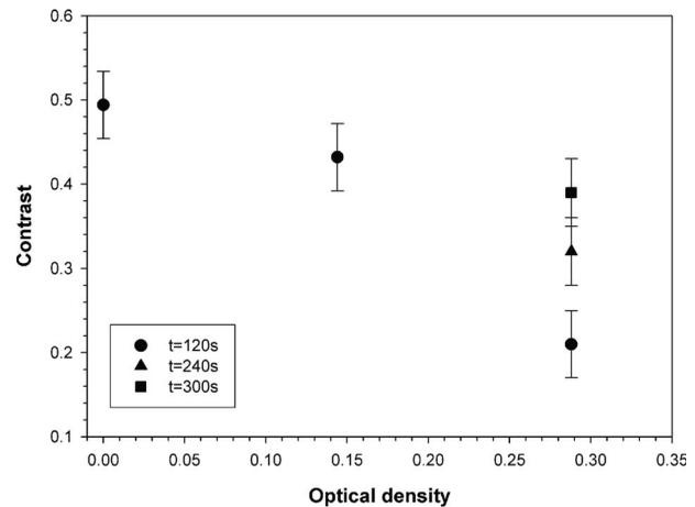
**Fig. 11** Shearographic fringe contrast recorded with the coupled system versus optical density for different scattering phantoms composed of silica spheres ( $d=611$  nm) in suspension in distilled water, as well as different hologram write times. Increased hologram write times can be seen to restore fringe contrast by restoring the spatial coherence of the input light to the shearographic interferometer.
