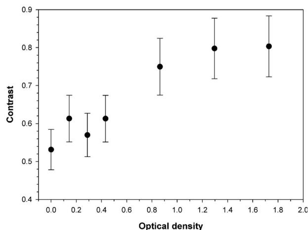
**Fig. 8** Hologram contrast versus optical density for different scattering phantoms composed of silica spheres ( $d=611$  nm) in suspension in distilled water.
