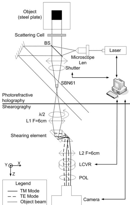
**Fig. 9** Schematic of the coupled experimental setup: photorefractive holography at the top and digital shearography at the bottom.
