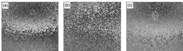
**Fig. 10** Three sheared holograms ( $5 \times 5$  median filtered) obtained with the coupled system. (a) Without a scattering cell, hologram write time of 120 s; (b) with a scattering cell ( $OD=0.288$ ), hologram write time of 120 s; (c) with a scattering cell ( $OD=0.288$ ), hologram write time of 300 s.
