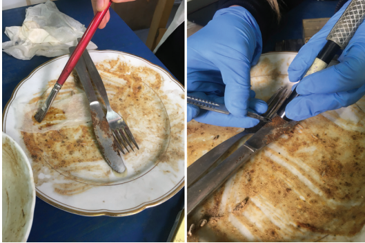
Fig. 2. Detail of the plate during the solvent cleaning (a) and the mechanical removal of the oxidation (b).
