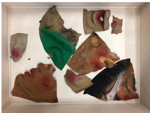
A vintage rubber mask after artificial aging processes. © J. Paul Getty Trust.
