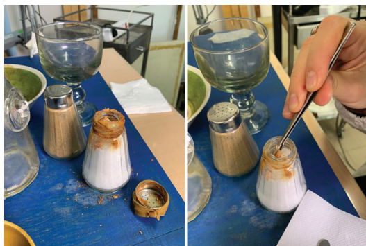
Fig. 3. Detail of the salt shaker after the opening (a) and during the rust salt removal (b).
