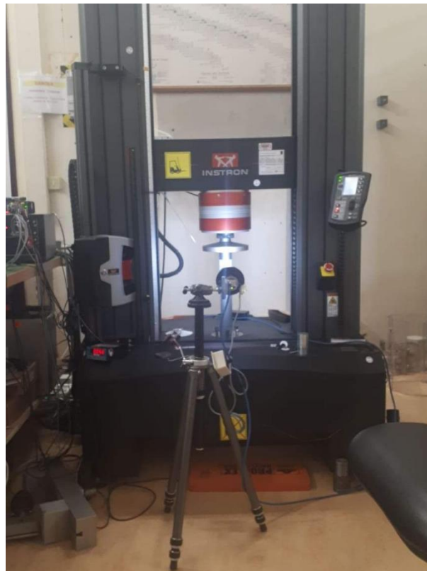
Fig. 4.12: Uniaxial compression device employed in LECBA (CEA) during the partnership ULG-CEA.
