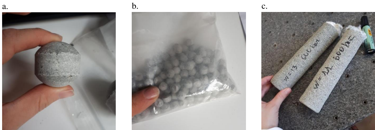
Fig. 5.1: MX-80 bentonite assemblies analysed in the experimental tests.
