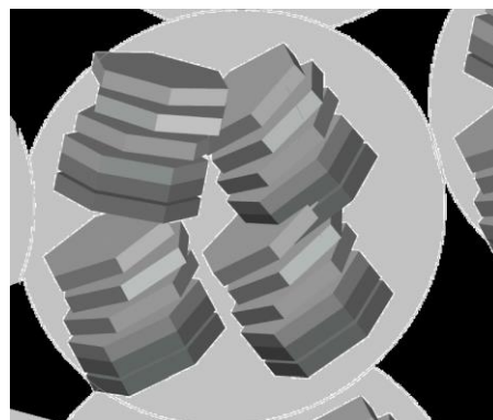
Fig. 2.8: Schematic representation of typical bentonite dry grain (modified after (Dor et al. 2020)). Tactoids (hexagonal structure), inter-tactoids porosity (grey) and inter-grains porosity (in black) are represented.
