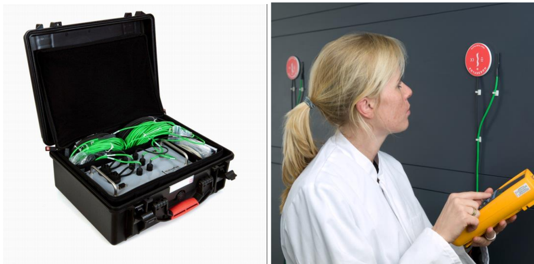
Fig. 4. HFP01 heat flux sensors in use on a wall.
