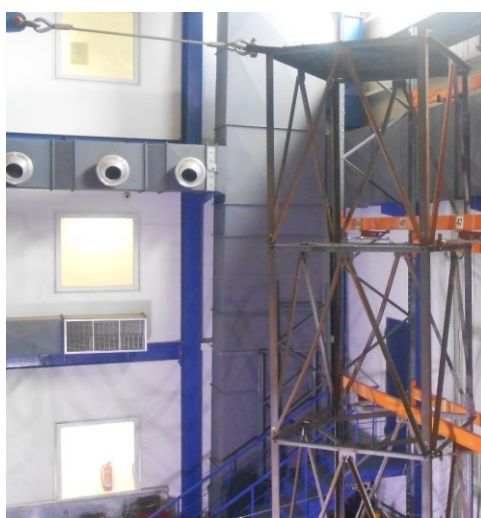
Figure 13.2: Tested tower with diagonal loading [51]
