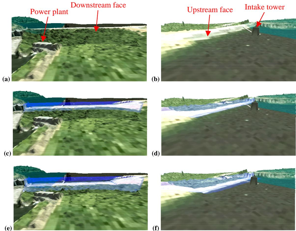
**Figure 5: 3D views of Eau d'Heure dam in the DEM (for 2D flow simulation) during the breaching.**
