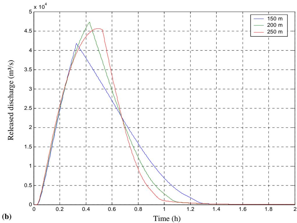
**Figure 7: Outflow hydrograph released at Eau d'Heure dam as a function of the breach width for a breach formation time either of 30 min (a) or adjusted according to the breach final width (b).**
