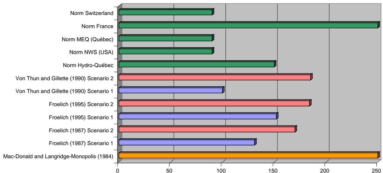
**Figure 3: Breach final width (m) according to empirical models and regulations.**
