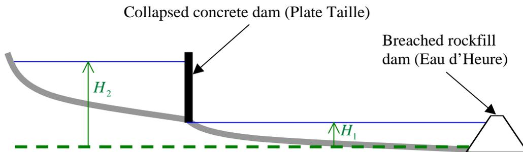
Figure 2: Schematic view of the two main reservoirs arranged in cascade.
