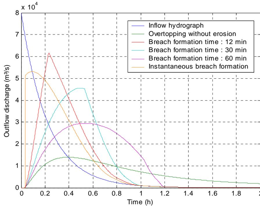
**Figure 6 : Hydrographs released at Eau d'Heure dam in the case of various breach formation times as well as in the case of an overflow without erosion of the structure.**
