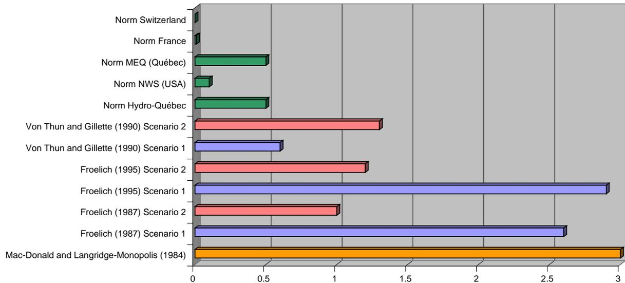
**Figure 4: Breach formation time (h) according to empirical models and regulations.**
