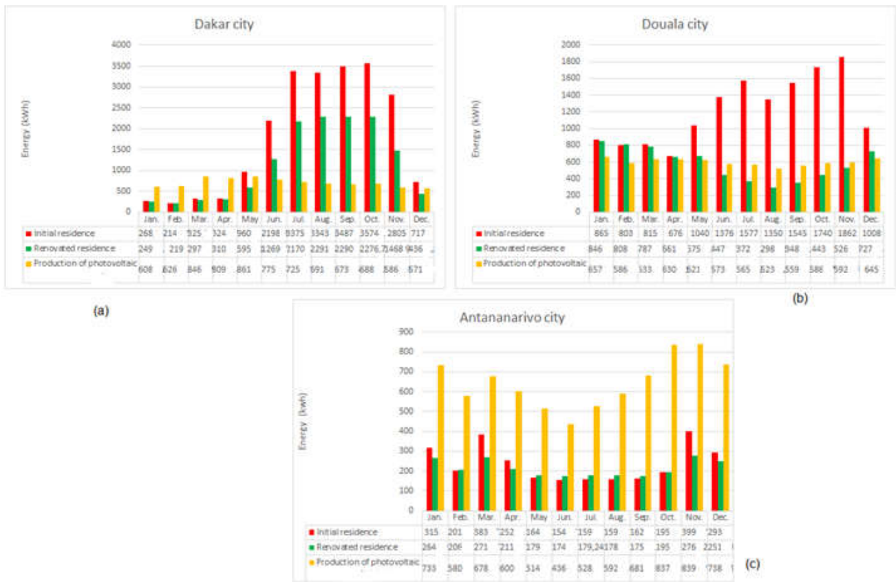
Figure 6. Monthly energy demand and production by photovoltaic panels in Dakar city (a); Douala (b); and Antananarivo (c).
