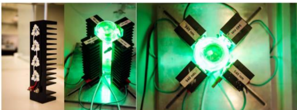
Fig. S13. Details of the irradiation setup for microfluidic photooxygenations
