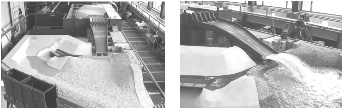
Figure 7: global scale model (left) and detailed study of the scouring intensity induced by the impinging jet downstream of the flip-bucket (right).
