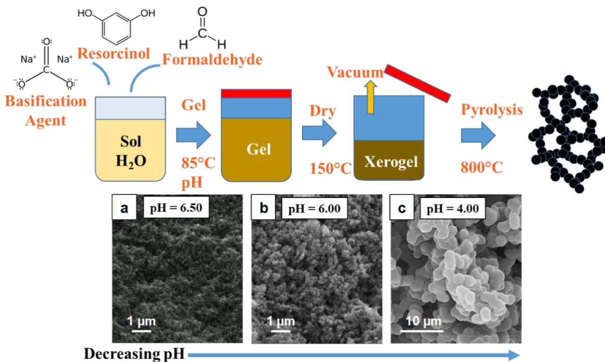
Figure 12 – Synthesis procedure for a resorcinol-formaldehyde carbon xerogel using \text{Na}_2\text{CO}_3 as a basification agent. Corresponding SEM images of the carbon xerogel morphology are shown when the pH of the precursor solution is changed [71].
