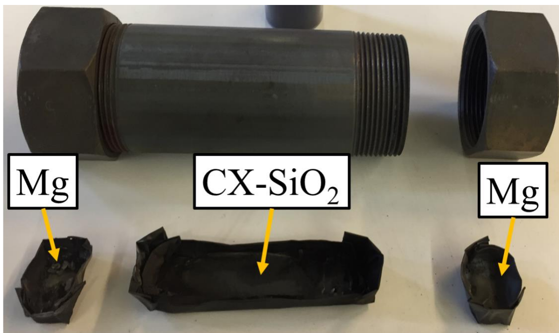
Figure 4.2 – Magnesiothermal reactor made of 304 stainless-steel. The sample holders for the magnesium chips and CX-silica samples were constructed out of 304 stainless steel foil.
