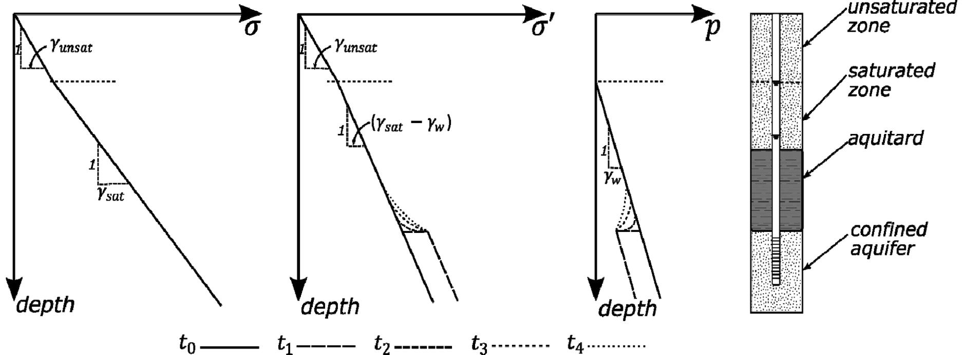
➔ **Land subsidence induced by pumping in confined aquifers is due mostly to a slow increase of effective stress in the compressible confining layers (above and below the pumped aquifer):**
