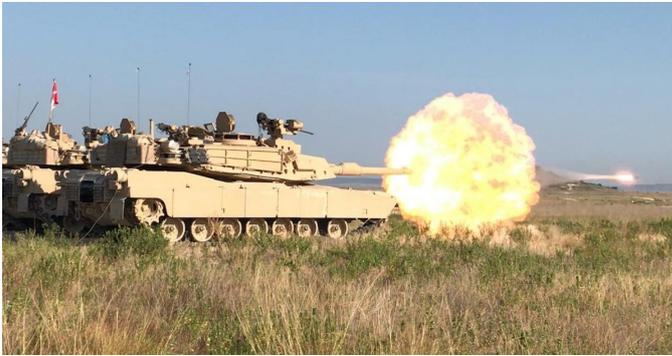
Figure 1.2: **Direct fire** - M1A2C Abrams tank with a 120-mm smooth bore.
