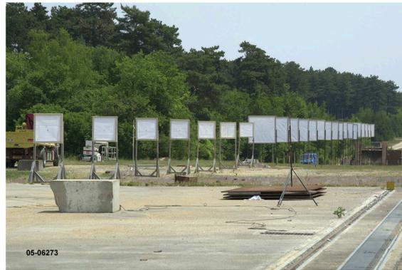
Figure 6.1: Yaw cards installed on the shooting range of Bourges (FRA) consisting of wooden posts between which are stretched sheets of kerosene, paper or cardboard, to disrupt the flight as little as possible [41, 52].
