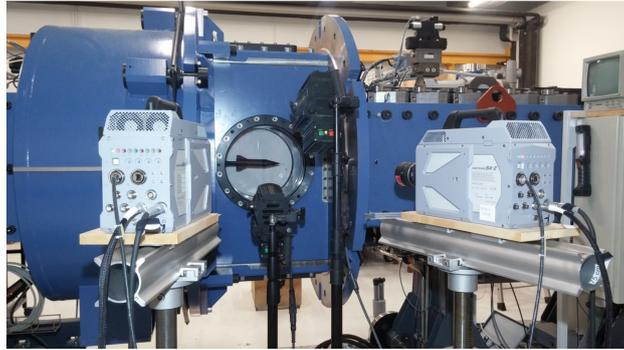
Figure 6.3: ISL's trisonic blow down wind tunnel with high speed camera's for stereovision-technique[134, 155].
