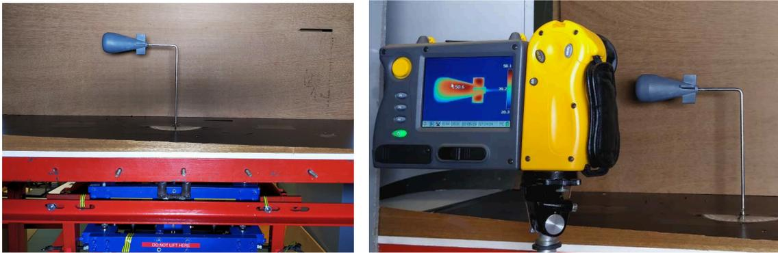
Figure 10.2: Left : Aerodynamic balance for drag, lift and pitch measurements. Right : IR FlexCam for the temperature profiles visualization.
