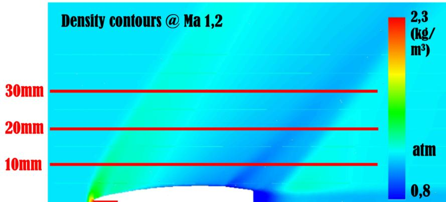
Figure 11.8: Numeric density contours with three parametric zones where the density was evaluated using the BOS technique on the .338-in. 300gr.-projectile.
