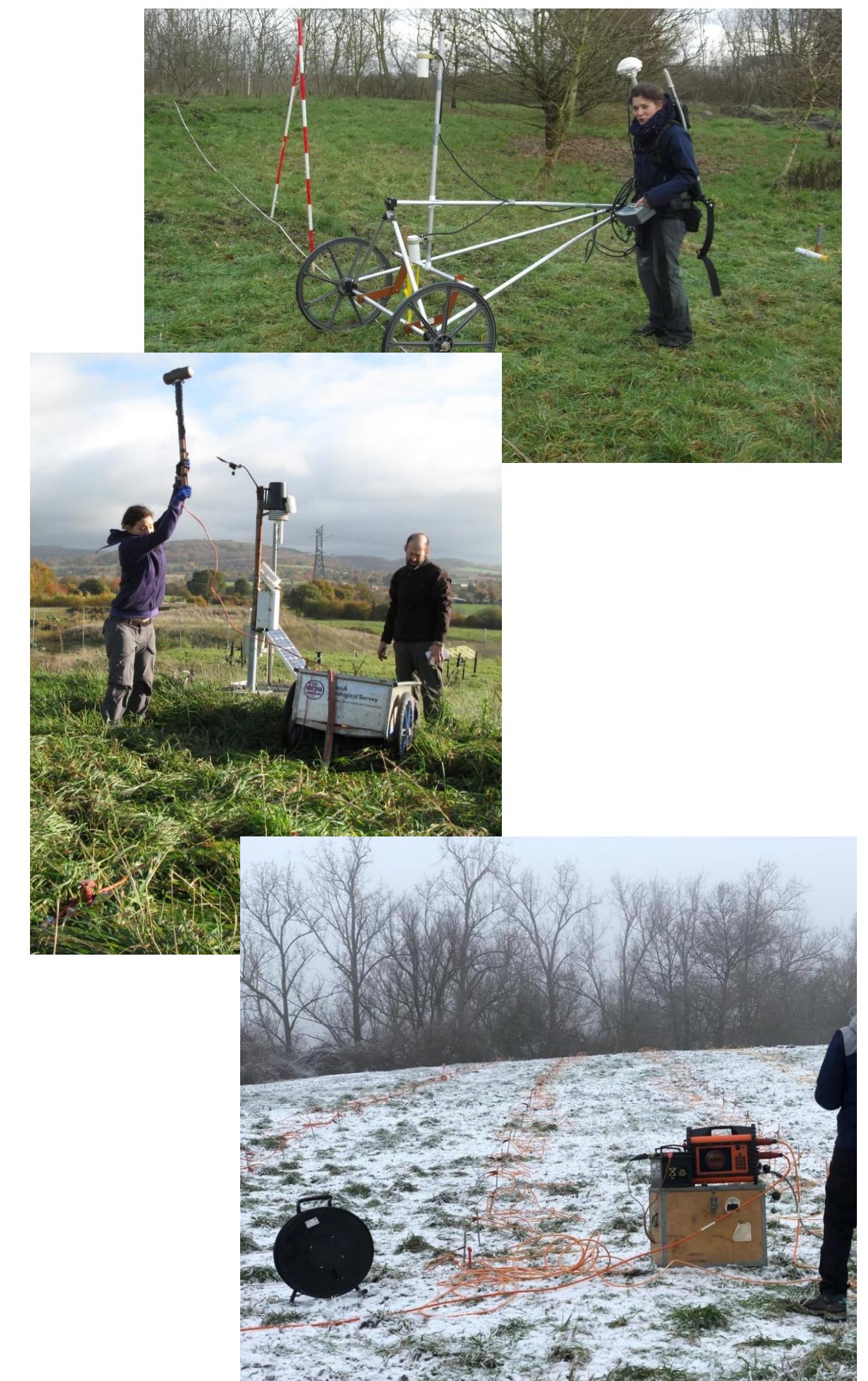
Fig. 4. Magnetometry (top), EMI (middle) and ERT/IP (bottom) acquisition.
