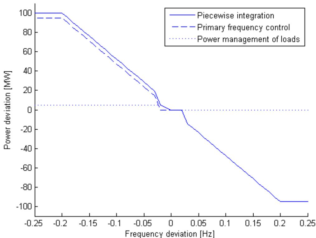
Figure 5.3: Power deviations for the piecewise integration
