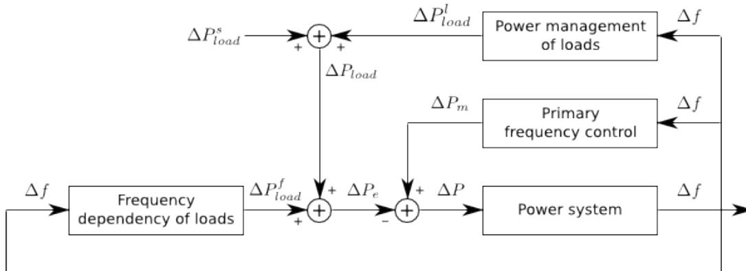
Figure 5.1: Block diagram of a power system with primary frequency control and with power management of loads
