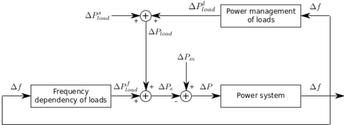
Figure 4.1: Block diagram of a power system with the power management of loads
