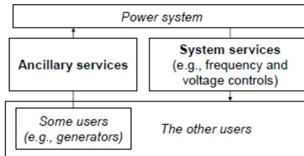
Figure 3.1: Distinction between ancillary and system services, taken from [Reb08]
