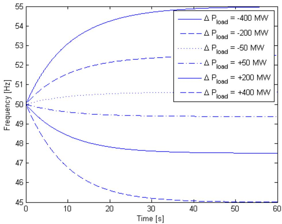
Figure 2.4: Theoretical frequency responses of uncontrolled power system, similar to [And11]
