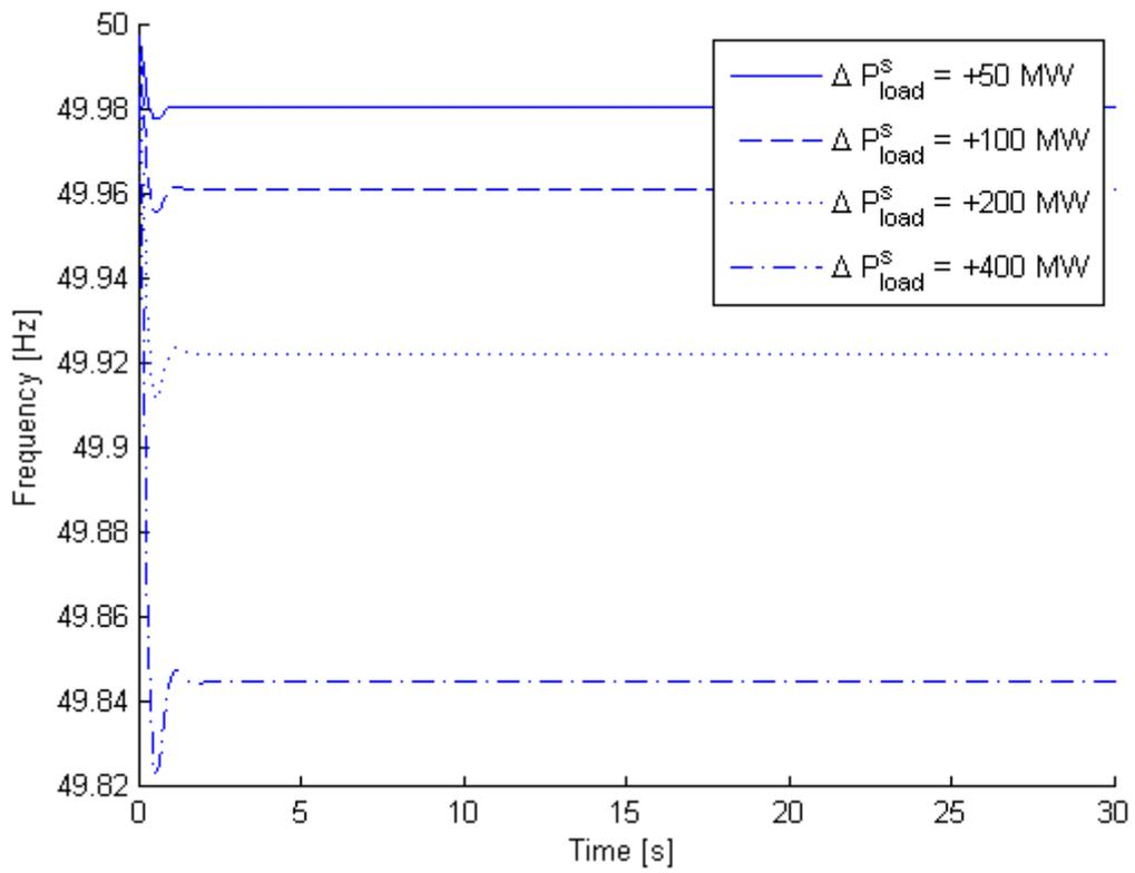
Figure 4.5: Theoretical responses of the power system with power management of loads, comparison on the load power deviation  $\Delta P_{load}^s$  with  $\tau = 0.2$  s and  $N_0 = 10^7$  loads.
