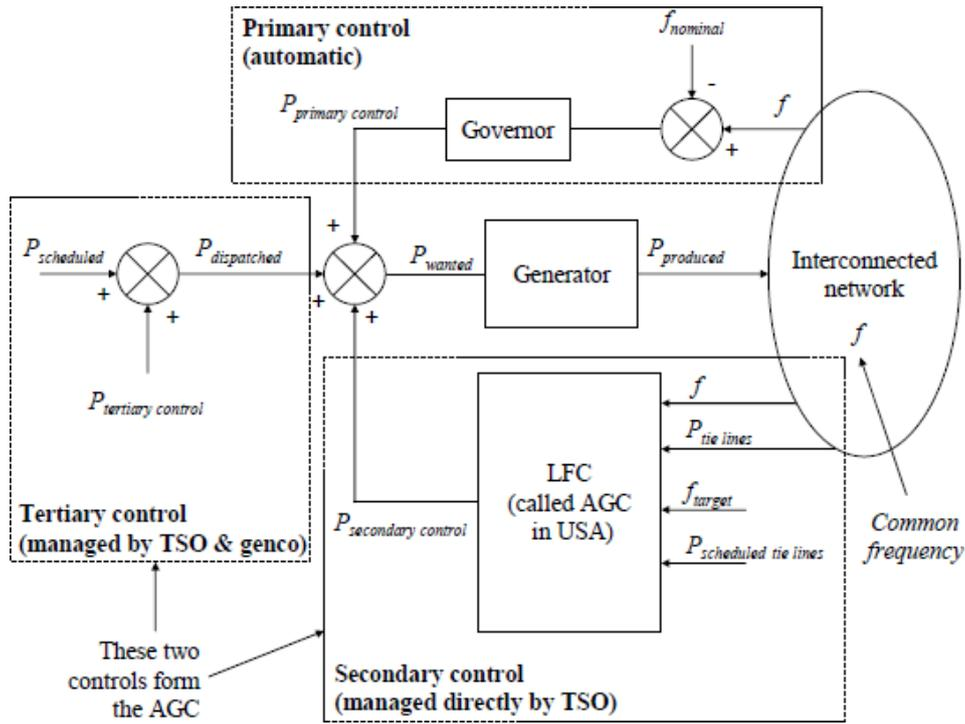
Figure 3.2: Framework for frequency control in Europe, taken from [RK05]
