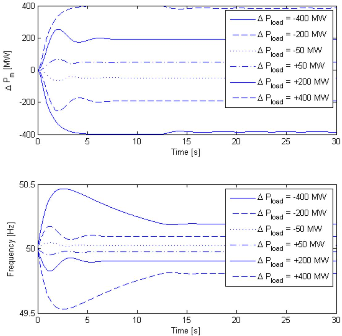
Figure 3.8: Theoretical responses of the power system with primary frequency control, comparison on  $\Delta P_{load}$  with  $\tau_t = 1$  s
