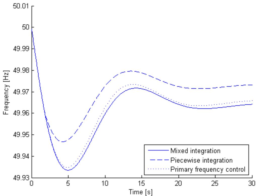
Figure 5.7: Comparison about theoretical responses for a power system with primary frequency control, with mixed integration and with piecewise integration, for  $\Delta P_{load}^s = +20$  MW and  $N_0 = 10^5$  loads
