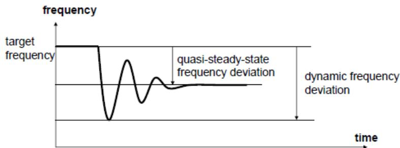
Figure 3.3: Dynamic and quasi-steady-state frequency deviation, taken from [Reb08]
