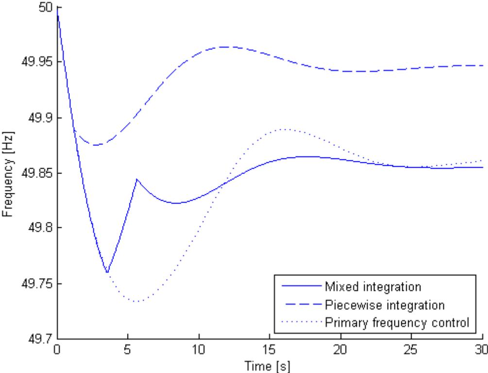
Figure 5.6: Comparison about theoretical responses for a power system with primary frequency control, with mixed integration and with piecewise integration, for  $\Delta P_{load}^s = +80$  MW
