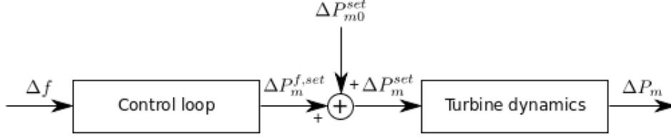
Figure 3.6: Block diagram of the primary frequency control
