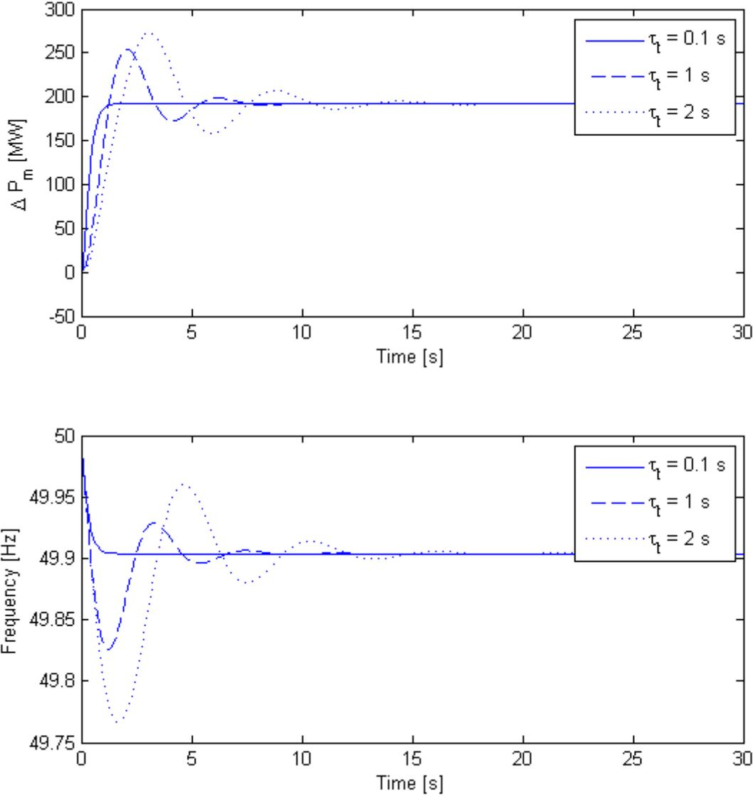
Figure 3.10: Theoretical responses of the power system with primary frequency control, comparison on  $\tau_t$  with  $\Delta P_{load} = +200$  MW
