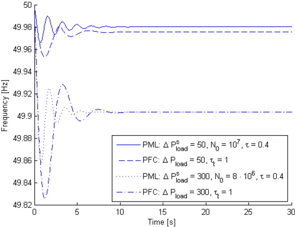
Figure 4.6: Theoretical responses to compare a power system with power management of loads (PML) and a power system with primary frequency control (PFC) with different primary reserves and with the same ones.
