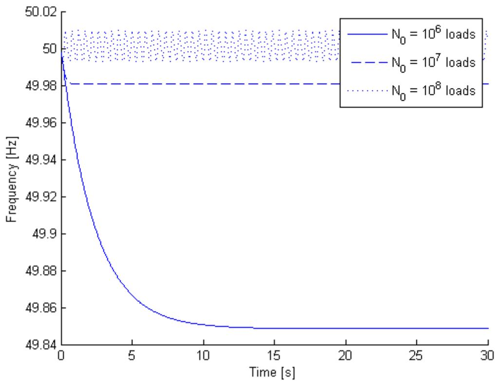
Figure 4.7: Theoretical responses of the power system with power management of loads, comparison on the available loads  $N_0$  with  $\tau = 0.1$  s and  $\Delta P_{load}^s = +50$  MW.
