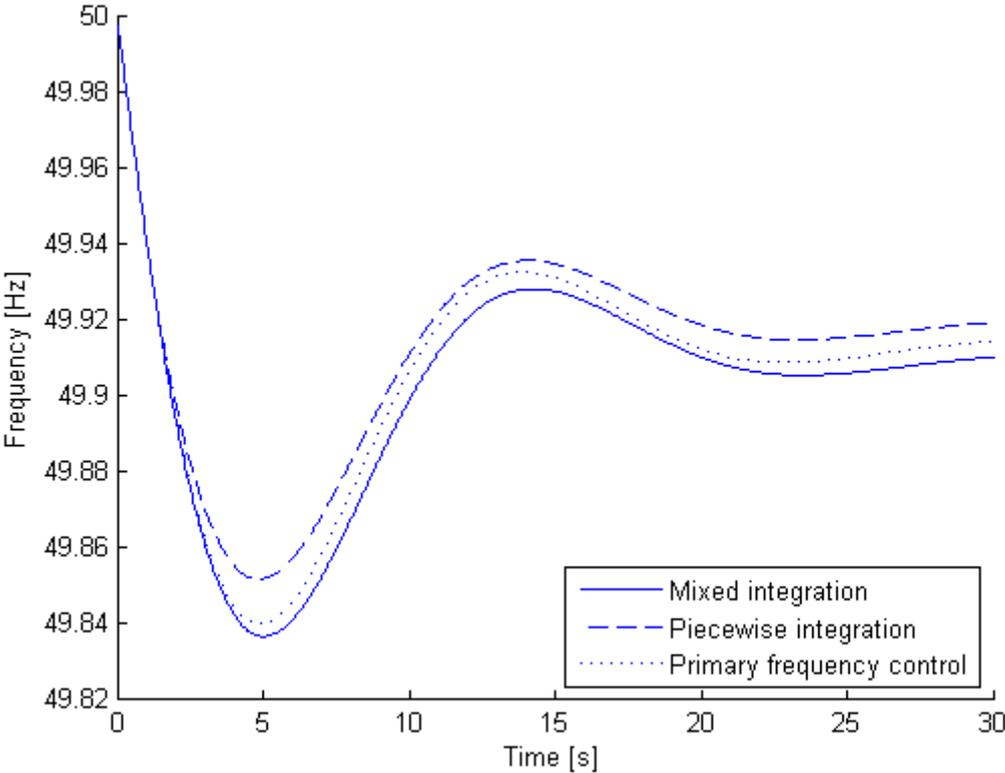
Figure 5.5: Comparison about theoretical responses for a power system with primary frequency control, with mixed integration and with piecewise integration, for  $\Delta P_{load}^s = +50$  MW and  $N_0 = 10^5$  loads
