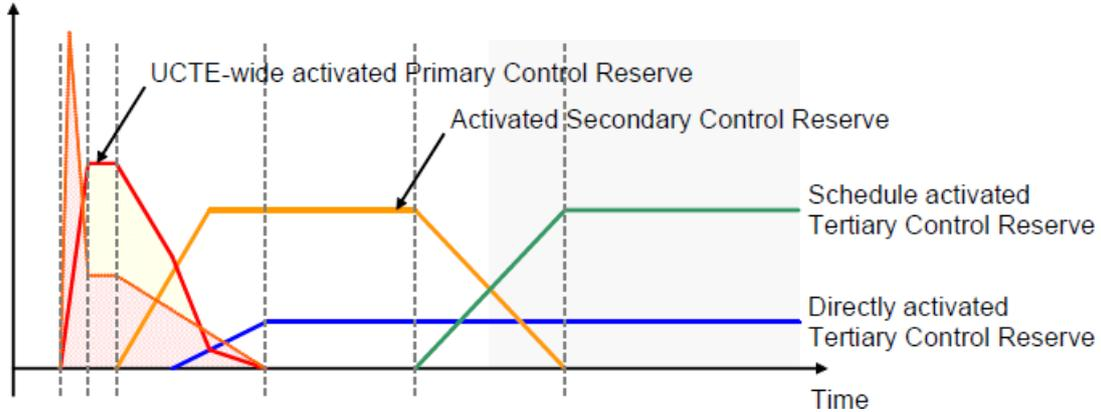
Figure 3.4: The frequency deviation and the activation of reserves, taken from [UCT09]
