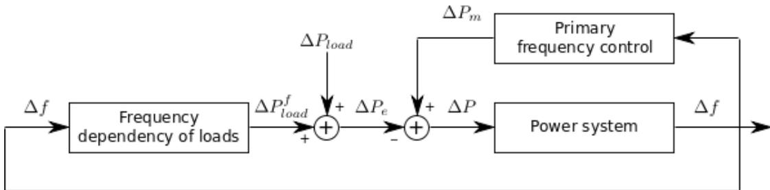
Figure 3.5: Block diagram of a power system with primary frequency control
