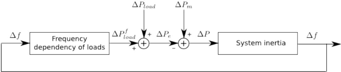
Figure 2.2: Block diagram of an uncontrolled power system
