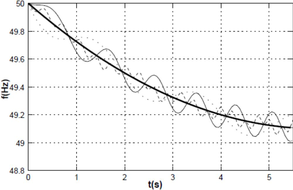
Figure 2.1: The system frequency and differences occurred for some generators, taken from [And11]
