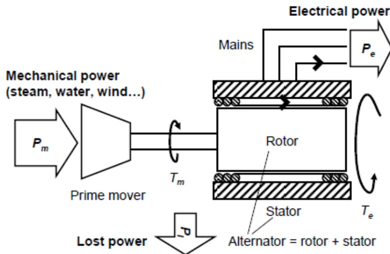
Figure 2.3: Principle of a synchronous machine as generating unit, taken from [Reb08]
