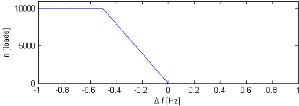
Figure 4.4: Example of a allocation function as a P-controller with  $N_0 = 10^4$  loads and  $\Delta f_{min} = -0.5$  Hz
