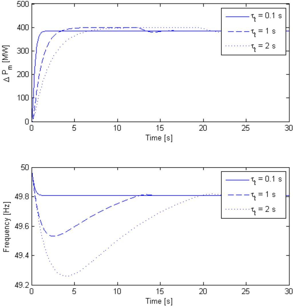
Figure 3.9: Theoretical responses of the power system with primary frequency control, comparison on  $\tau_t$  with  $\Delta P_{load} = +400$  MW
