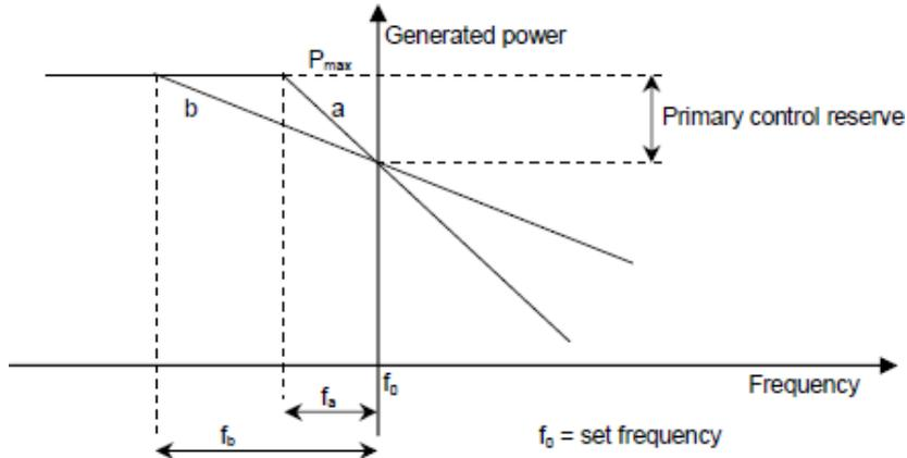
Figure 3.7: Graphical display of the speed droop characteristic, taken from [Ges10]
