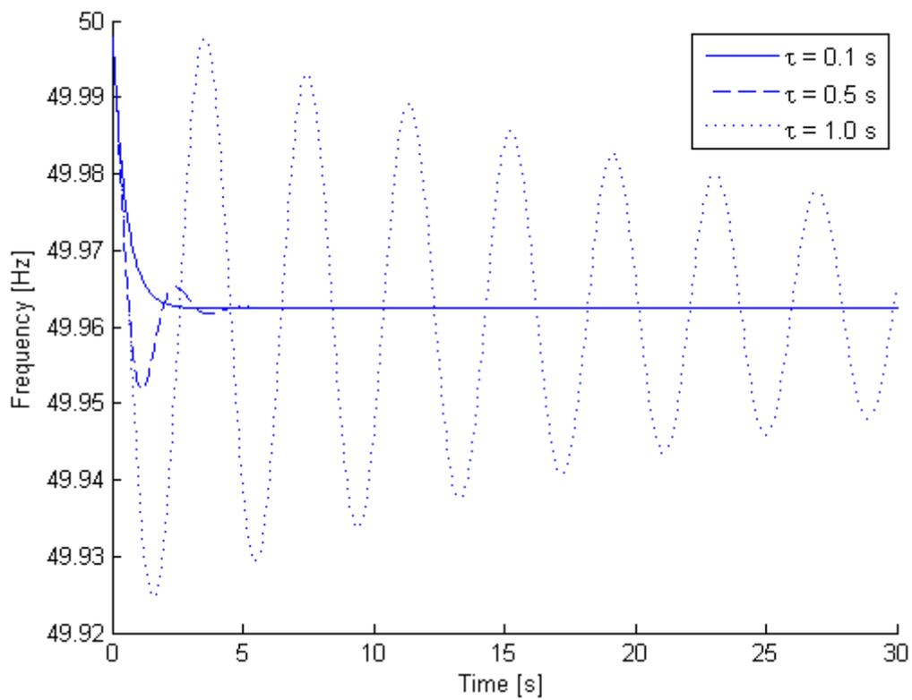
Figure 4.8: Theoretical responses of the power system with power management of loads, comparison on the time-delay  $\tau$  with  $\Delta P_{load}^s = +50$  MW and  $N_0 = 5 \cdot 10^6$  loads.
