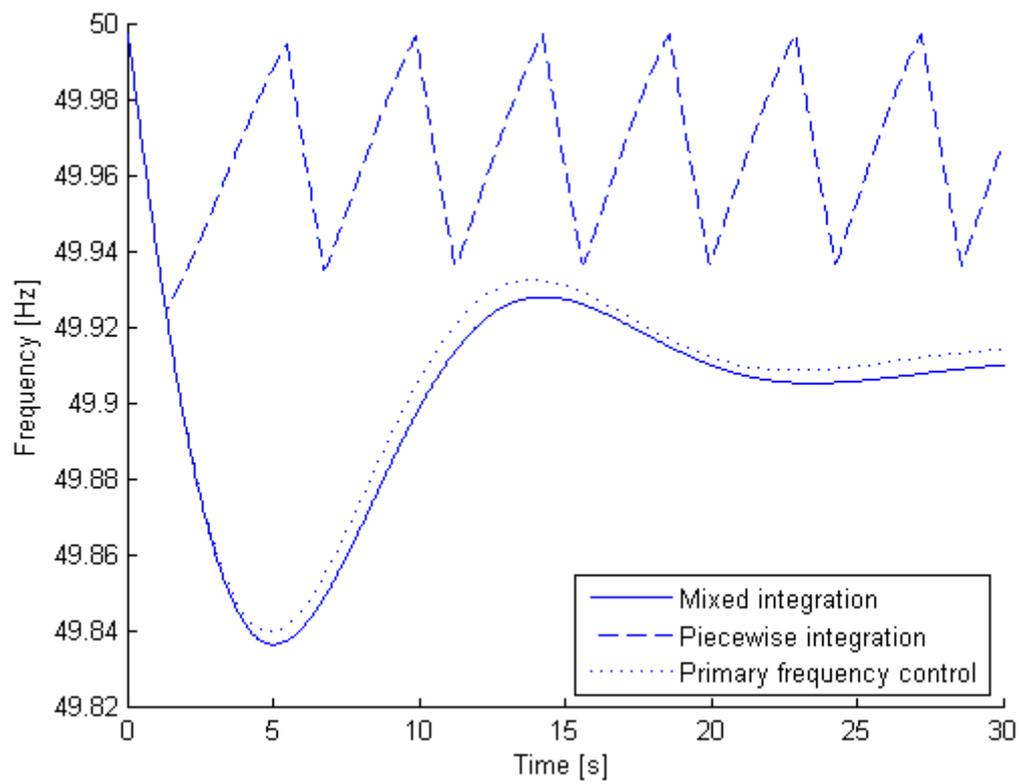
Figure 5.4: Comparison about theoretical responses for a power system with primary frequency control, with mixed integration and with piecewise integration, for  $\Delta P_{load}^s = +50$  MW
