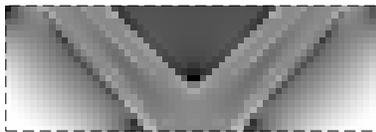
Figure 5: Homogenized von Mises stress for a minimum density of 1.e-1
