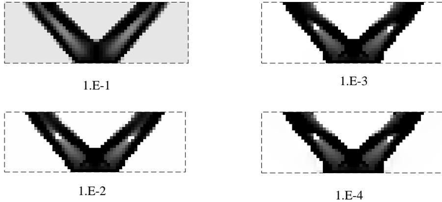
Figure 4: Topology designs with decreasing  $\rho_{min} = \epsilon^2$  parameters: 1.e-1, 1.e-2, 1.e-3, 1.e-4
