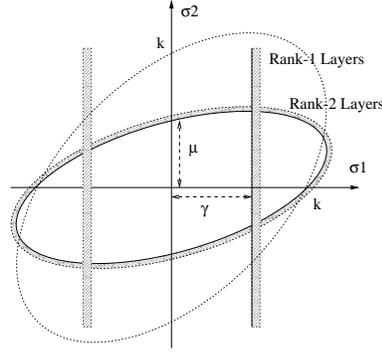
Figure 1: Overall strength domain of a rank 2 layered materials
