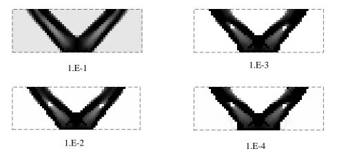
Figure 4: Topology designs with decreasing  $\rho_{min} = \epsilon^2$  parameters: 1.e-1,1.e-2, 1.e-3, 1.e-4
