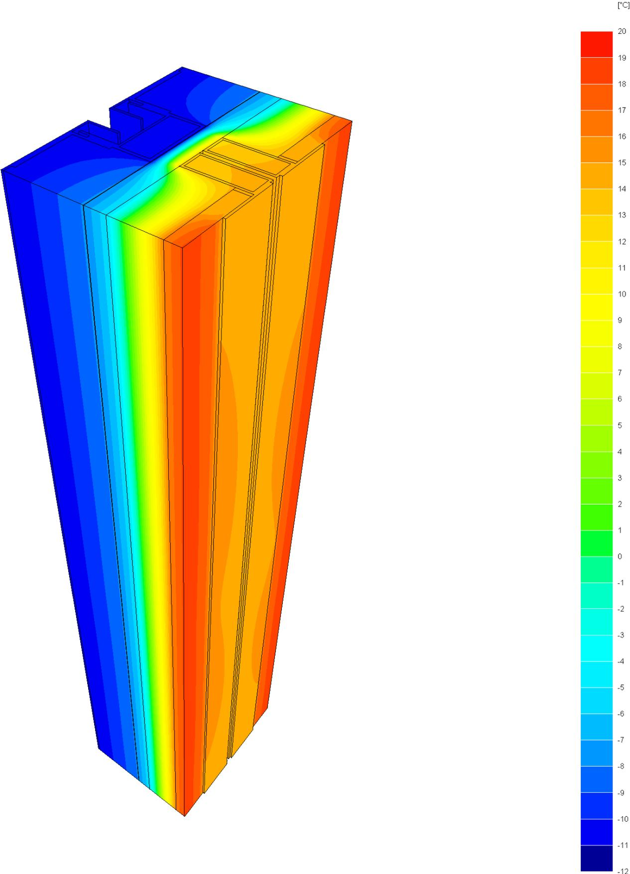
As expected, the aluminum and steel structures are the weakness in the thermal profile. Their high lambda value reflects the fact that they are excellent thermal conductors: the isothermal lines seem to get closer between those frames.
