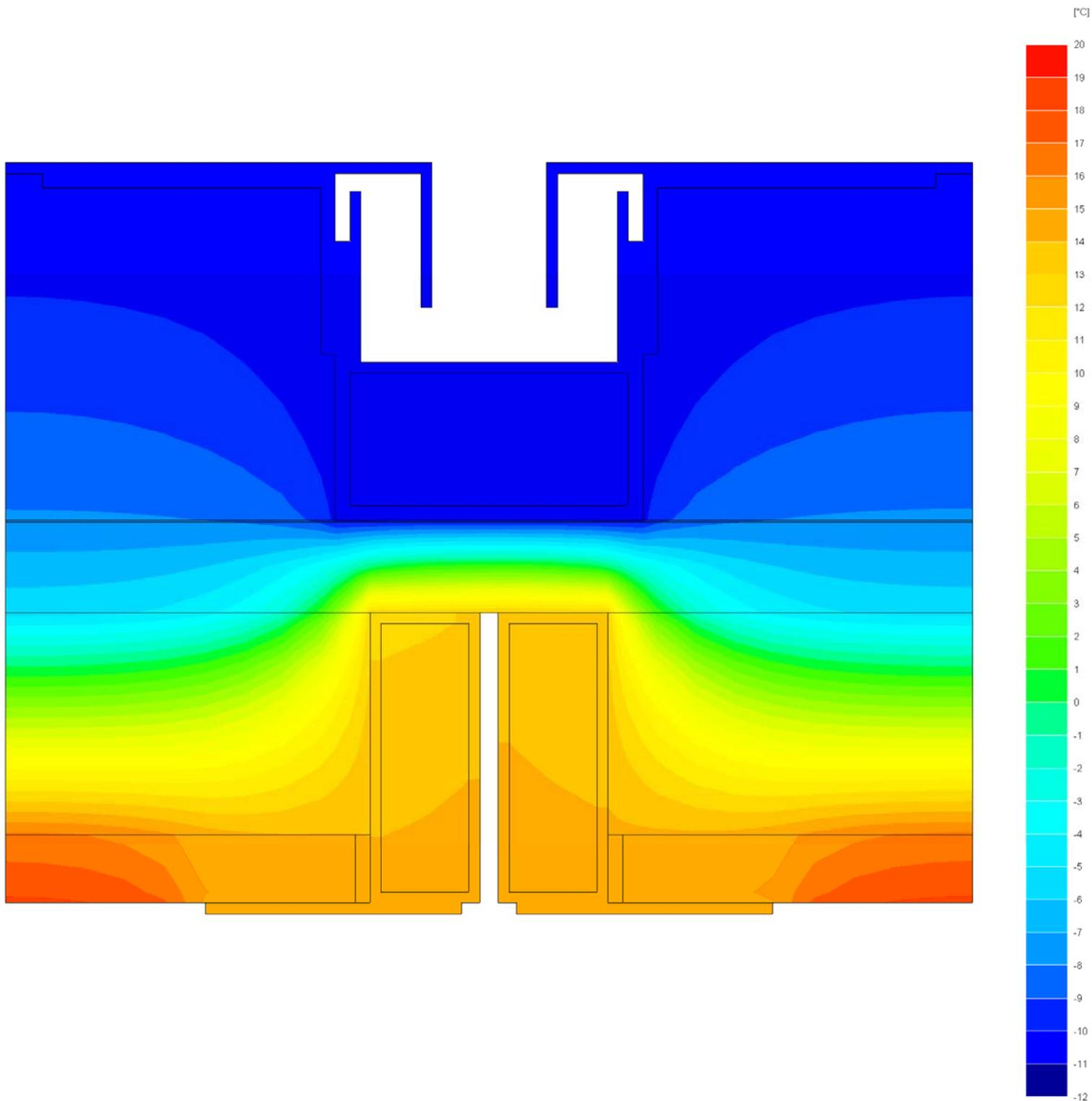
This first temperature profile is the one we can find almost all along the structure (where there is no bolt to break the symmetry). We can see that, for the temperatures given for boundary conditions, the symmetry is almost perfect, and the temperatures are spread in a range from  $-11^{\circ}\text{C}$  on the external face to  $14^{\circ}\text{C}$  to  $19^{\circ}\text{C}$  on the internal face.
