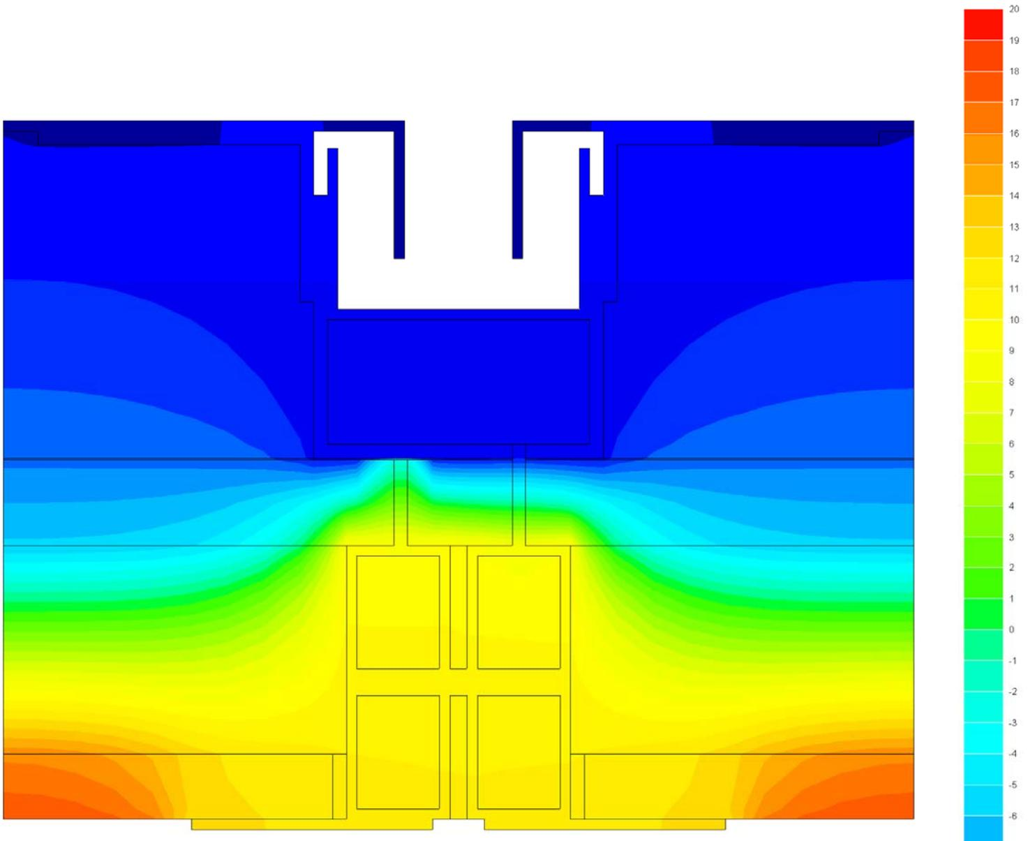
This profile at bolts section confirms what has been said previously: the presence of the POM reduces the minimal inside temperature, from 14°C to about 10°C.
