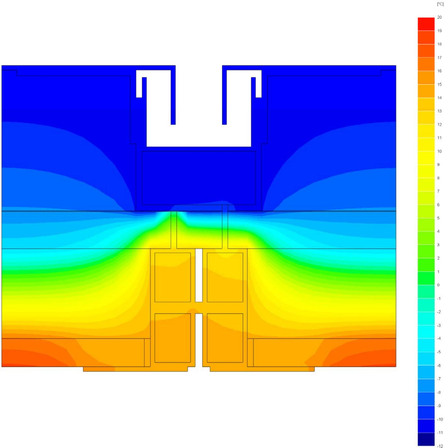
This profile is the one at the bolt section. One of these bolts crosses the aluminum frame, whereas the other one does not. This induces a small asymmetry on the profile.
