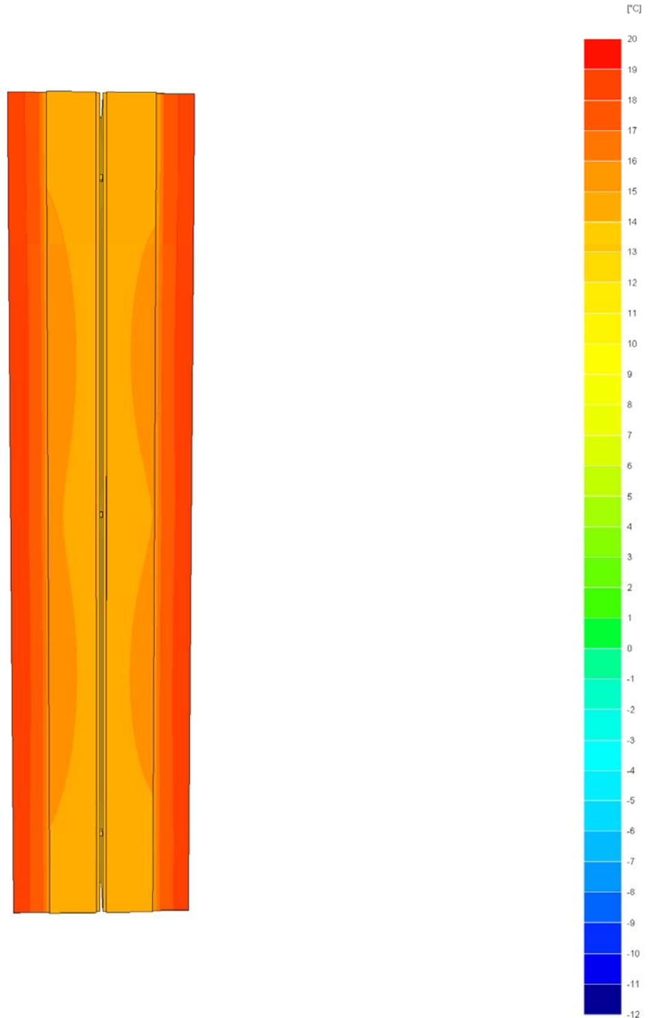
The temperature range we can notice is from 14 to 19°C. But we can find a lower temperature between the steel frames (about 12°C).
