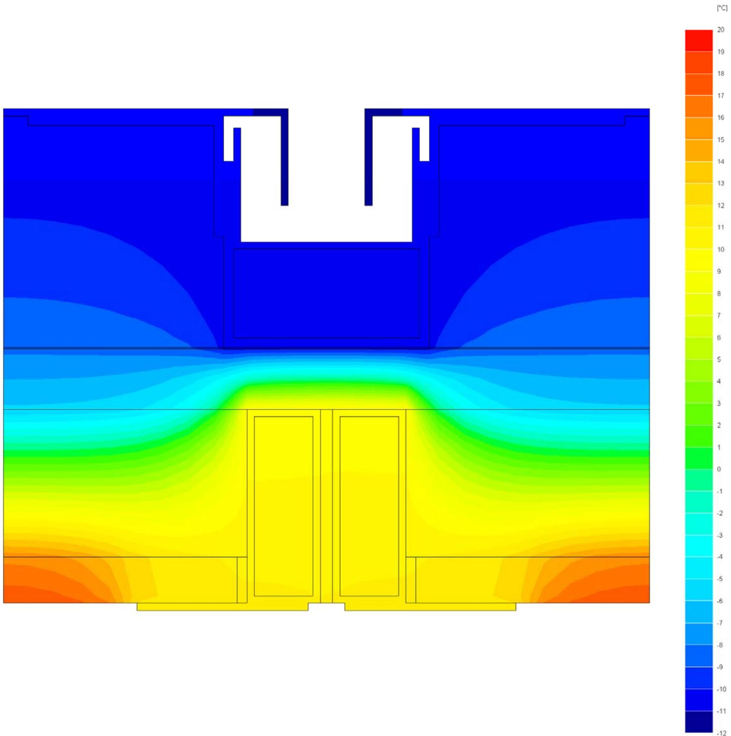
We can see that the results are even getting worse with that additional material filling the gap. The reason seems quite simple: in the previous model, that space used to be filled with 20°C air (h=8). Now, it is filled with a material surrounded by steel at a lower temperature: the POM will get to this temperature, and bring those results: the temperature of the inside faces of the model are lower than in the previous basic model, going from 10 to 17°C (instead of 14 to 18°C).
