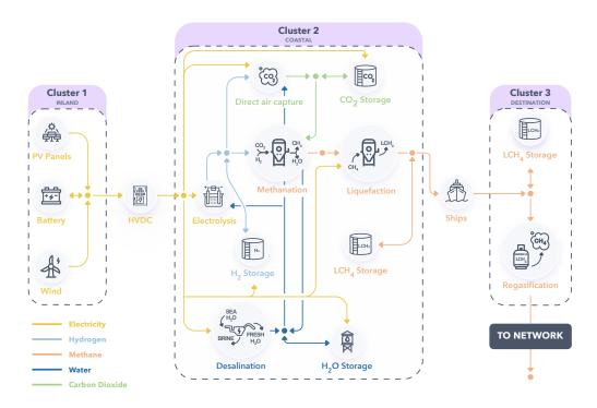
Figure 4: Remote carbon-neutral fuel supply chain [1]. Icons represent conversion and storage nodes, while bullets and arrows schematically represent hyperedges.
