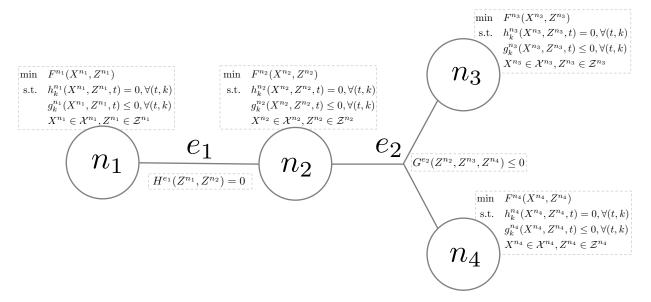
Figure 1: Graph abstraction of a hypothetical problem whose block structure is represented by four nodes (i.e.,  $\mathcal{N} = \{n_1, n_2, n_3, n_4\}$ ) and two hyperedges (i.e.,  $\mathcal{E} = \{e_1, e_2\}$ , with  $e_1 = \{n_1, n_2\}$  and  $e_2 = \{n_2, n_3, n_4\}$ ). Note that  $e_1$  only has equality constraints while  $e_2$  only has inequality constraints in this example.
