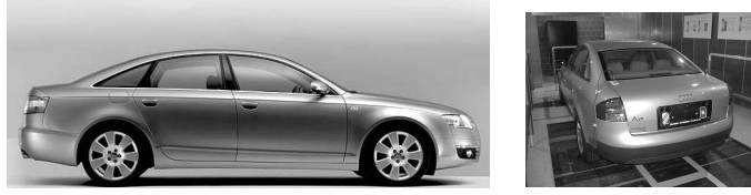
Figure 1: Audi A6 (left) and the same vehicle on 4 poster rig for testing and its instrumentation with corner accelerometers (right).
