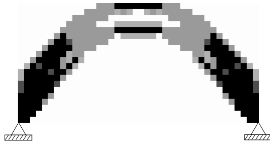
Figure 27: Topology obtained by CONLIN at iteration 200
