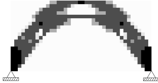
Figure 26: Topology obtained by CONLIN at iteration 199
