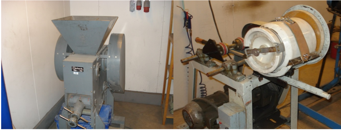
Figure 58 : Jaw crusher (left) and Ball mill (right) used in this work
